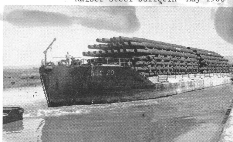
BOUND FOR ANCHORAGE is a barge loaded with pipe from Napa-Fab. The large-diameter pipe will be used to construct a deep water pier in the tide-troubled port.
