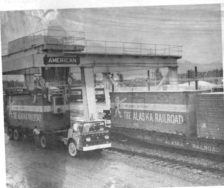
THE ALASKA RAILROAD 40-ton gantry crane expedites unified defense transport service. Here, military-bound freight, in URB (Unit Rail Box) traveled by ocean freight to Seward, and was transhipped via rail to Anchorage. In the background is Fort Richardson, near Chugach Range.
