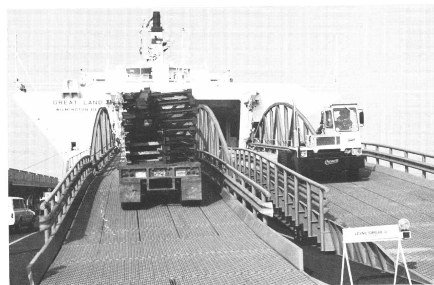
Loading operations in full swing at Terminal 37, Seattle. A trailer with a load of steel trusses is hauled up on the left ramp, while a tractor comes down the other ramp to pick up another trailer.
