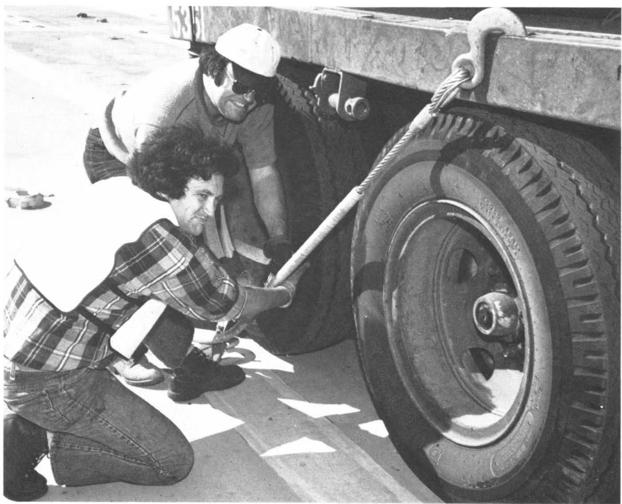
The upper photo shows a tractor being disengaged from a Roloc box after parking a trailer. The Roloc box is made secure by a lockdown button, while at the aft end of the trailer (bottom photo), turnbuckles are tightened to hold the load down.
