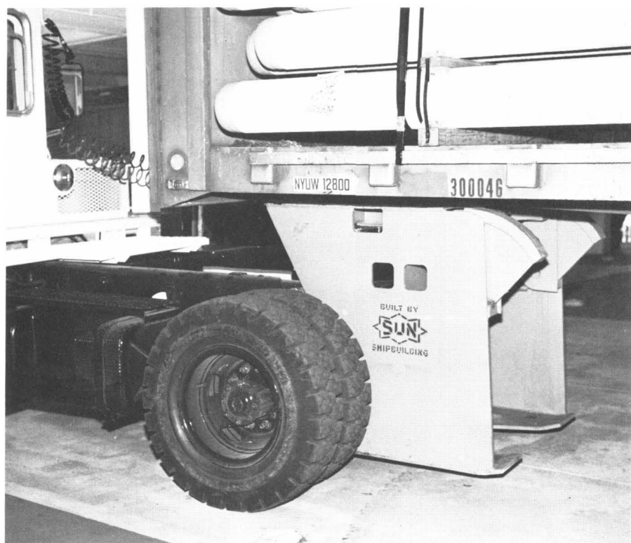
The upper photo shows a tractor being disengaged from a Roloc box after parking a trailer. The Roloc box is made secure by a lockdown button, while at the aft end of the trailer (bottom photo), turnbuckles are tightened to hold the load down.
