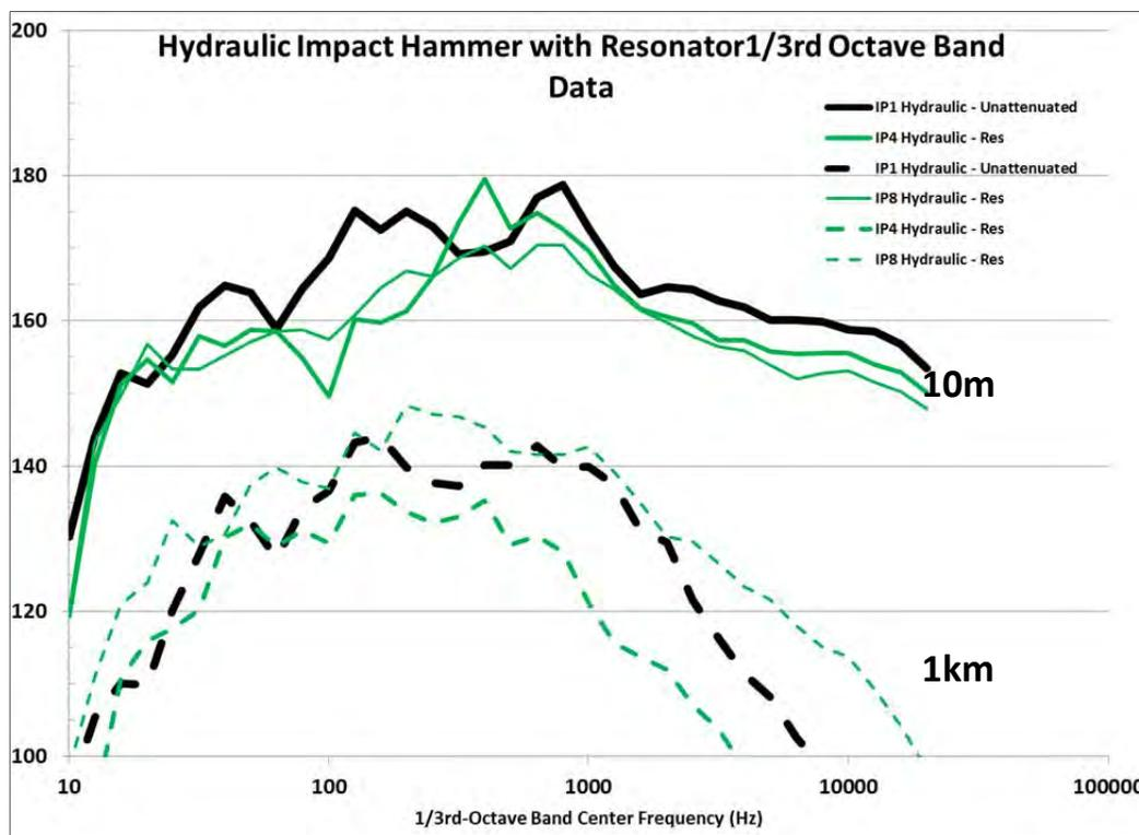
Figure 16. Median 1/3rd-octave band levels measured at 10 m and 1 km using the hydraulic impact hammer with Resonator.
