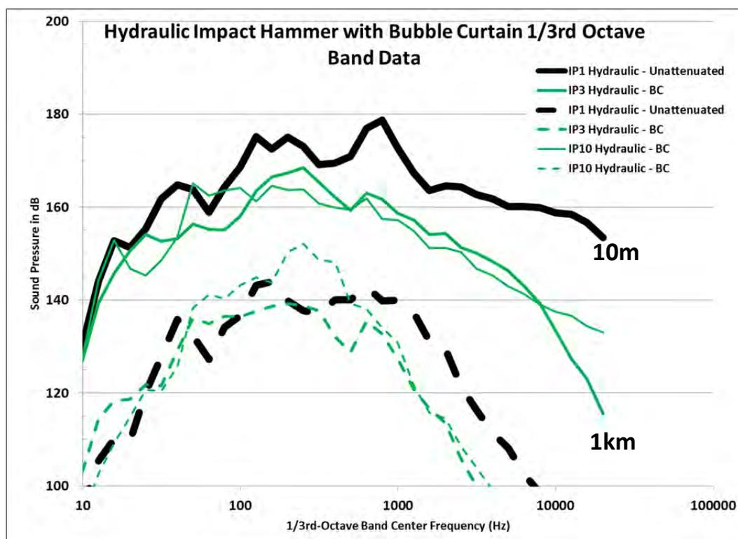
Figure 13. Median 1/3rd-octave band levels measured at 10 m and 1 km using the hydraulic impact hammer with air bubble curtain.
