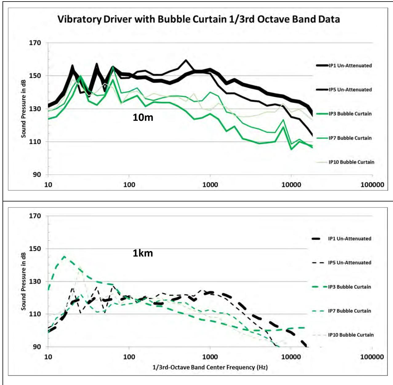
Figure 14. Median 1/3rd-octave band levels measured at 10 m (top) and 1 km (bottom) using the vibratory driver with air bubble curtain.
