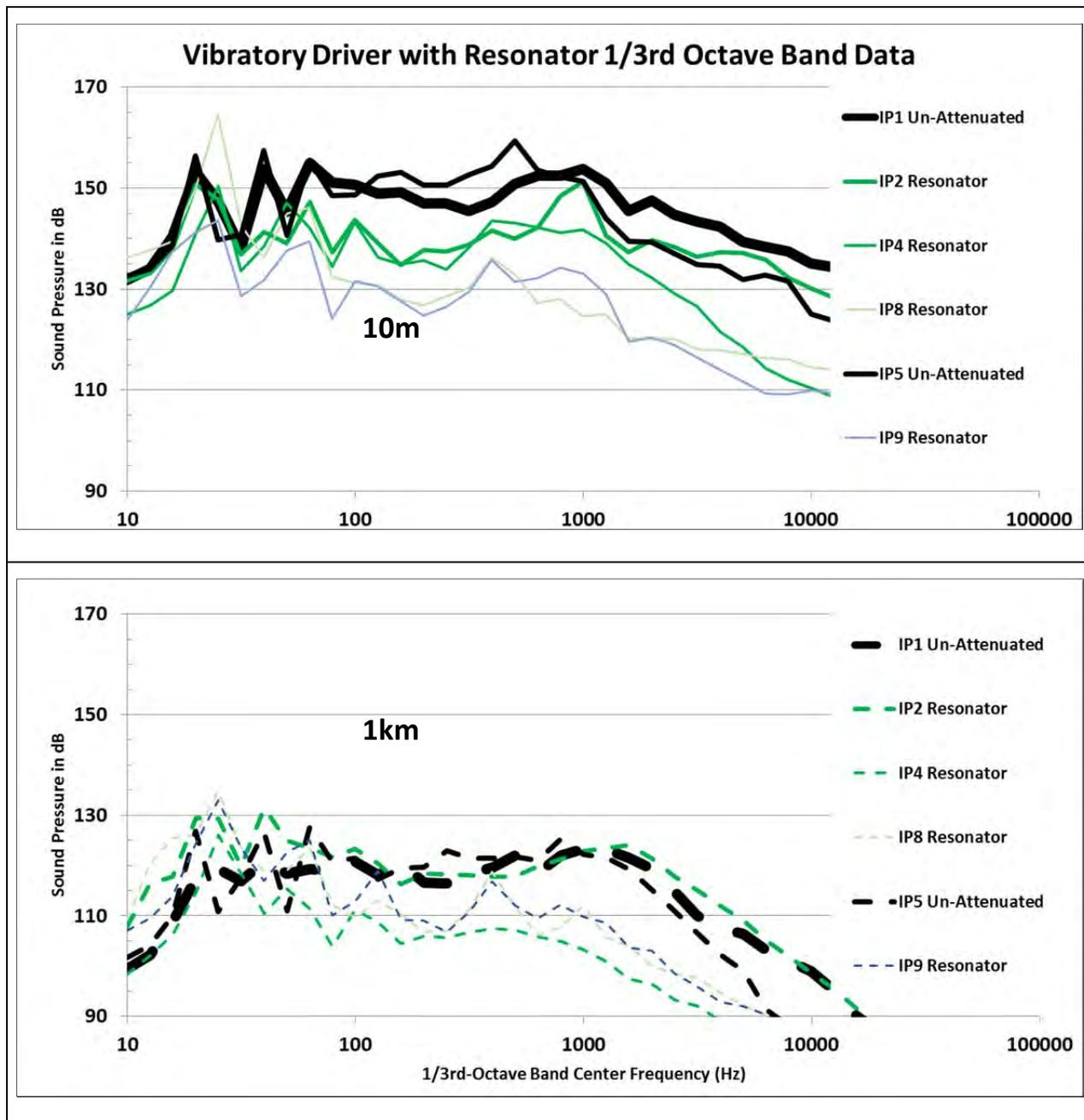
Figure 17. Median 1/3rd-octave band levels measured at 10 m (top) and 1 km (bottom) using vibratory driver with the Resonator.
