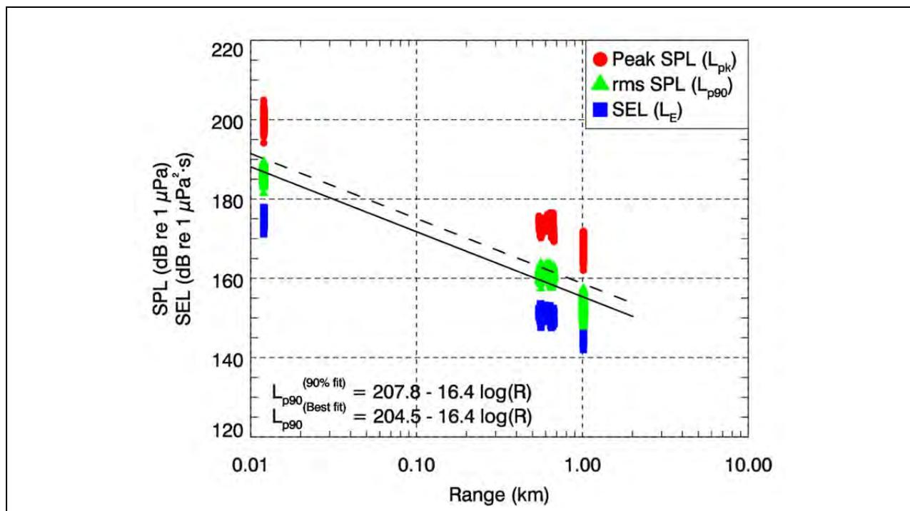
Figure 10. Pile IP7: Plot of peak SPL, RMS SPL, and SEL versus range for diesel impact driving.
