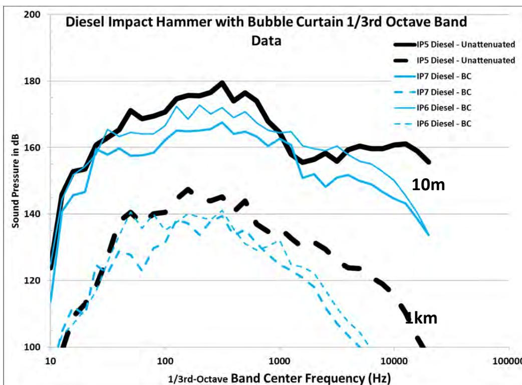
Figure 11. Median 1/3rd-octave band levels measured at 10 m and 1 km using the diesel impact hammer with air bubble curtain.
