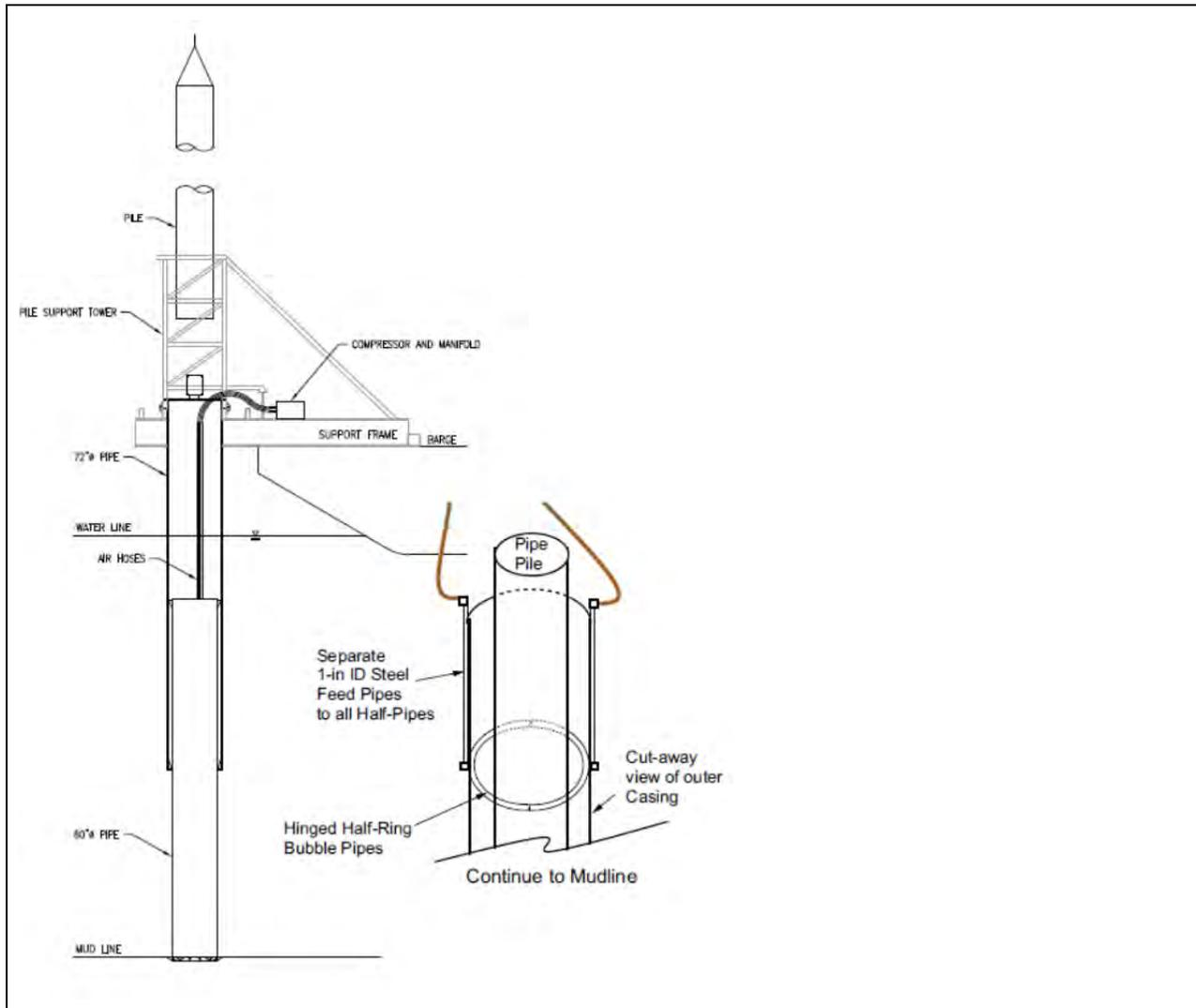
Figure 3. Confined bubble curtain system schematic.
