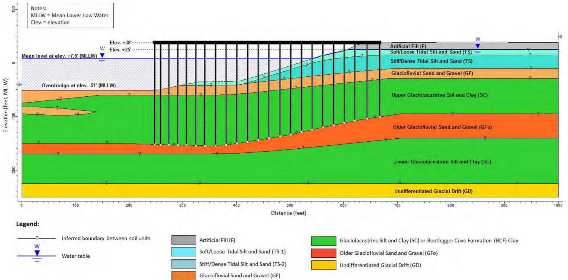
Figure 9. Typical soil cross section of Terminal 2 wharf and access trestle.
