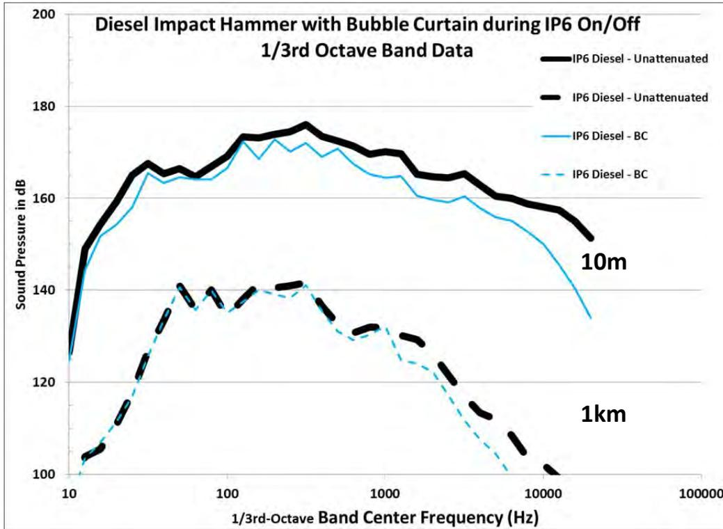
Figure 12. IP6 air bubble on and off test median 1/3rd-octave band levels measured at 10 m and 1 km using the diesel impact hammer.
