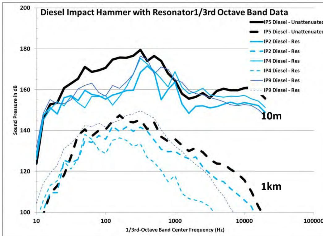
Figure 15. Median 1/3rd-octave band levels measured at 10 m and 1 km using the diesel impact hammer with resonator.
