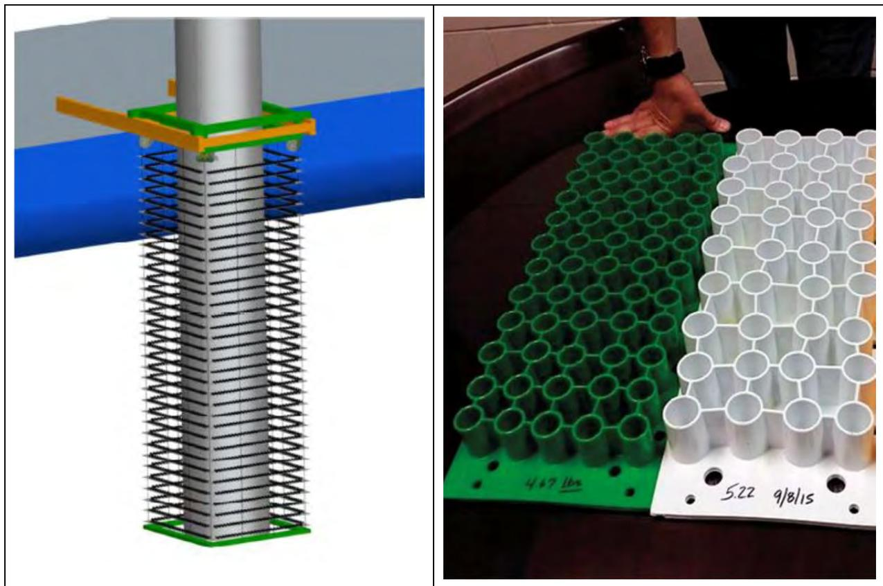
Figure 5. Schematic of deployed AdBm Passive Resonator system (left) and Helmholtz resonators (right). The open ends of the resonators face downward when deployed.
