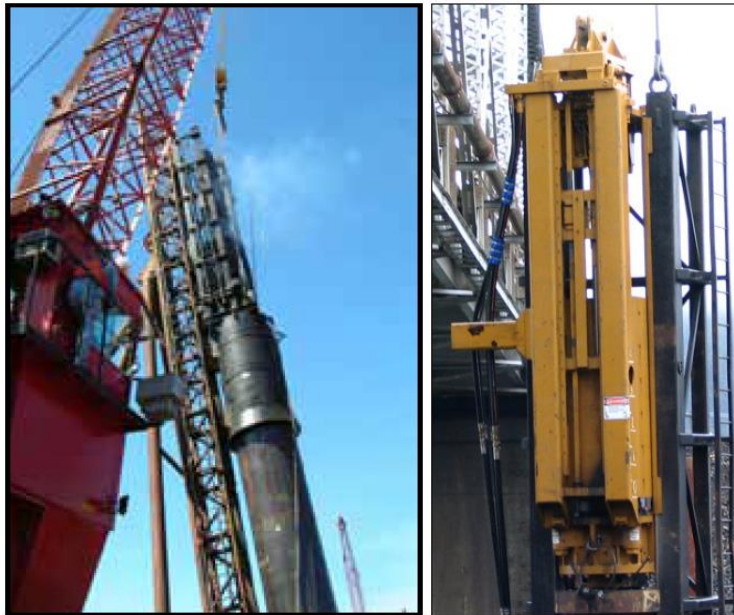
Figure 2. APE D-180-42 diesel impact hammer (left) and APE model 15-4 hydraulic impact hammer (right).
