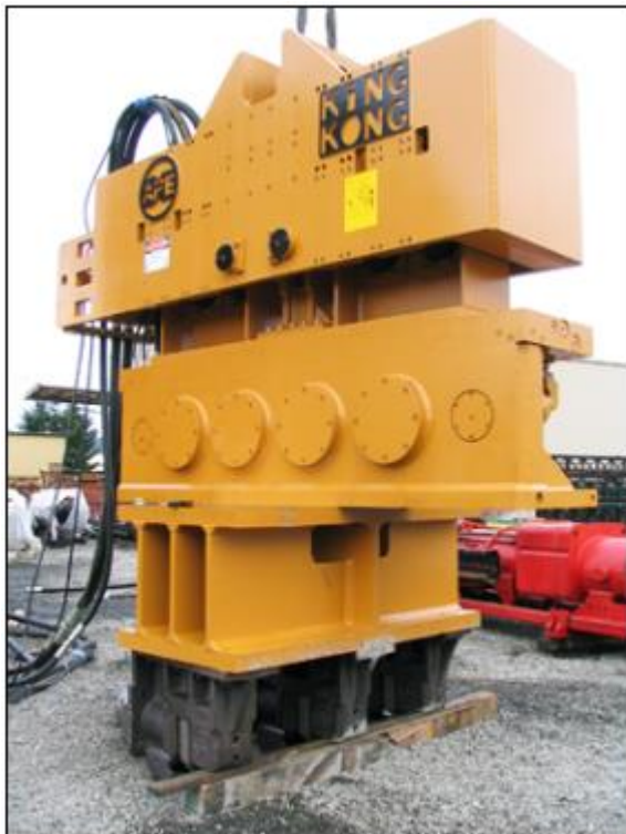
Figure 3. APE model 400 vibratory driver.
