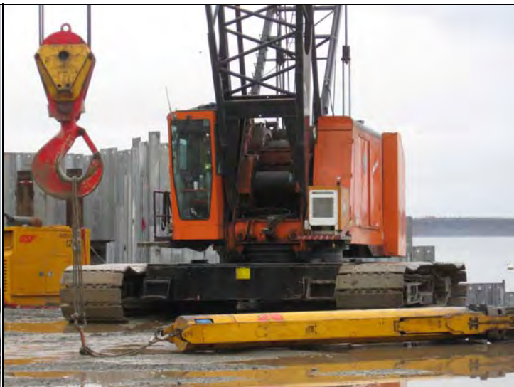
North Pad, South end at departure – 4100w Orange Tip idle, BSP SL30 impact hammer idle on ground
