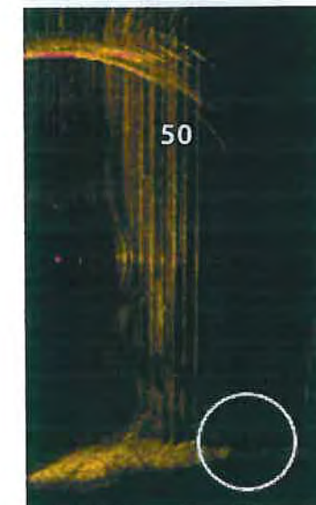
Interlocks on sheets appear to be straight and without gaps. The circled images along the mud line indicate an anomaly near the location that the divers discovered 18" from the pile walls and approximate location of sheet 11.
