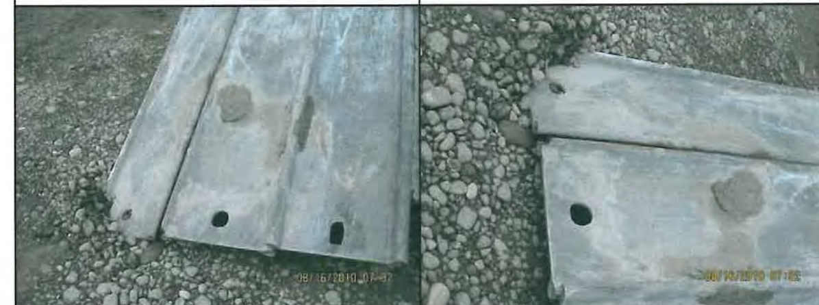
Separated interlock at tip of sheets.
