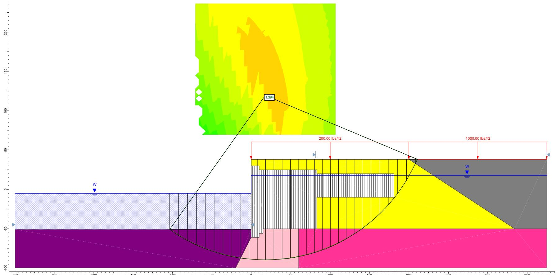
**Figure E25.** Re-analyzing the long-term static-undrained case for Section F using Slide (3-clay, circular surface).
