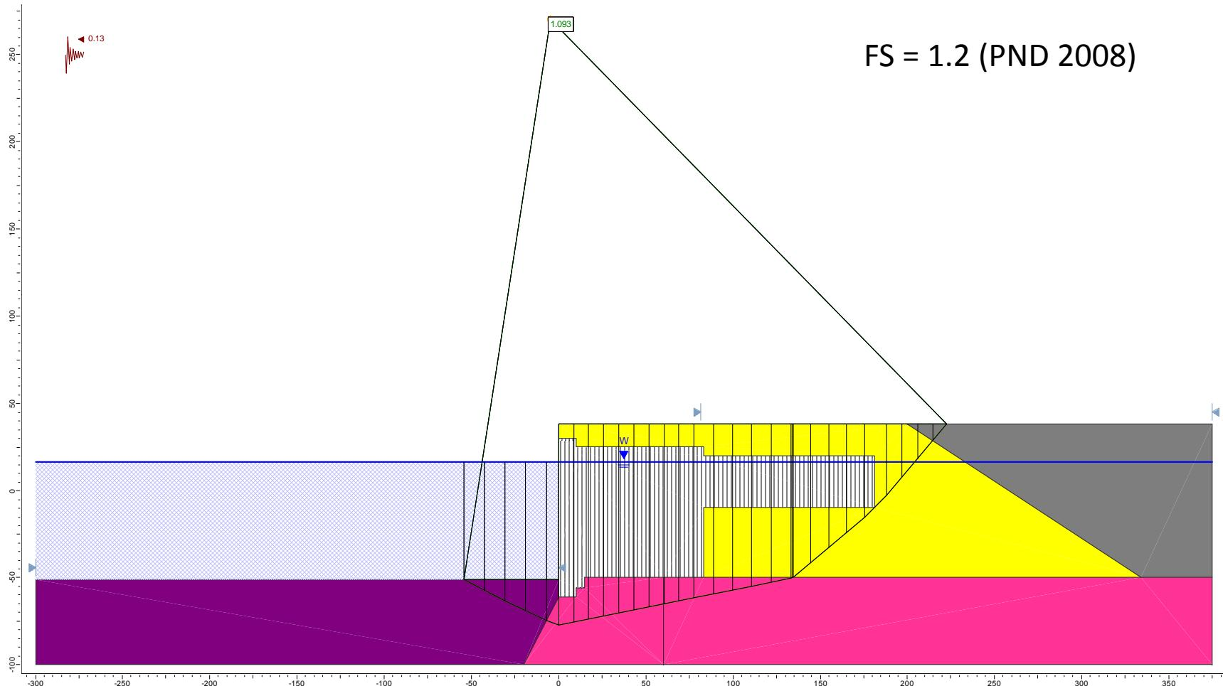
**Figure E48.** Re-analyzing the MCE case for Section F using Slide (2-clay, optimized surface).
