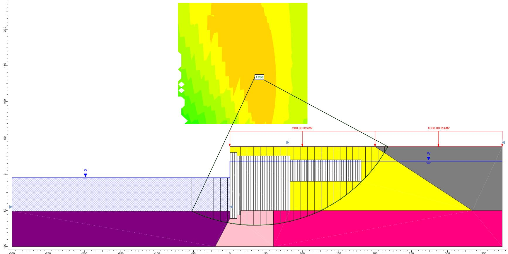
**Figure E17.** Re-analyzing the short-term static (EOC) case for Section F using Slide (3-clay, circular surface).
