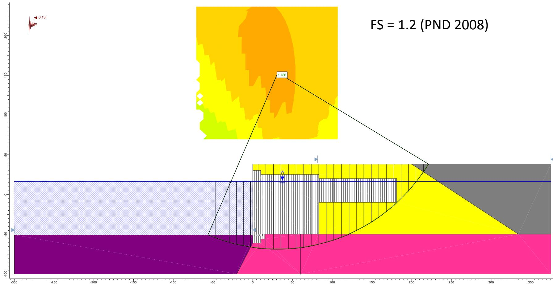
**Figure E47.** Re-analyzing the MCE case for Section F using Slide (2-clay, circular surface).
