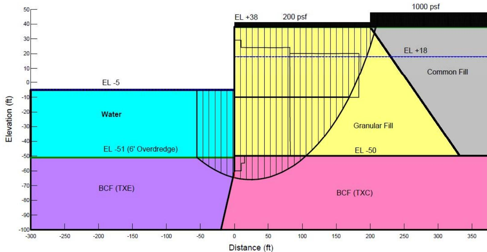
**Figure E7.** SLOPE/W model of Section F in short-term (EOC) and long-term static loading conditions (PND, 2008).
