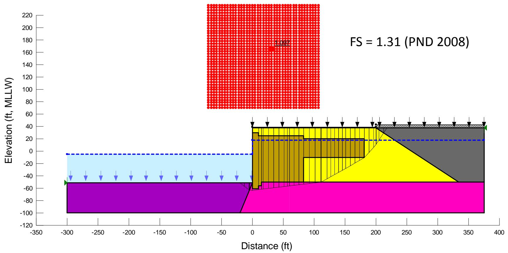
**Figure E12.** Re-analyzing the short-term static (EOC) case for Section F using SLOPE/W (2-clay, optimized surface).
