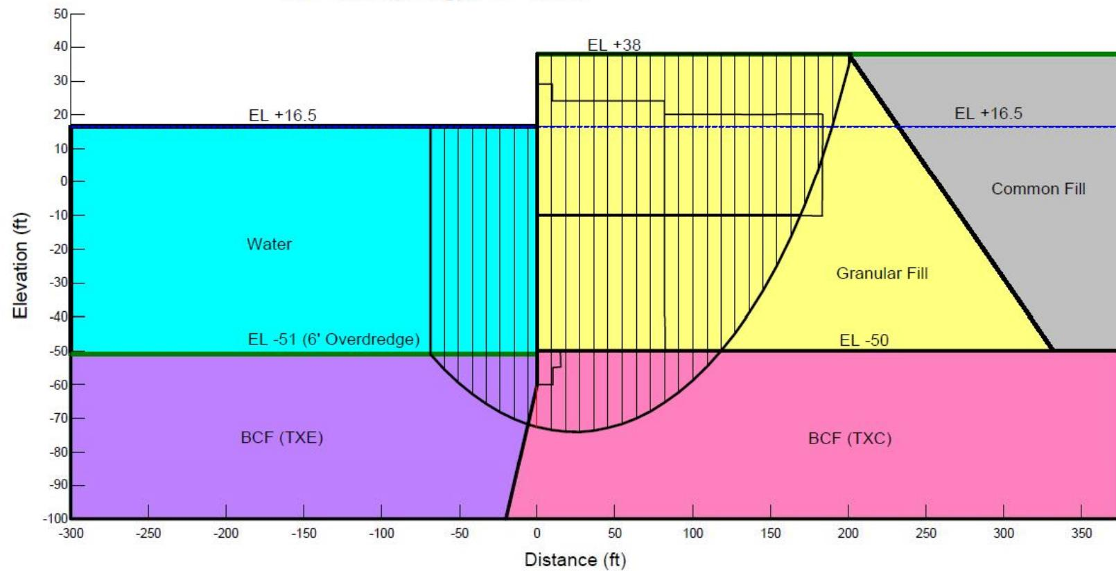
**Figure E8.** SLOPE/W model of Section F in pseudo-static loading condition (PND, 2008).
