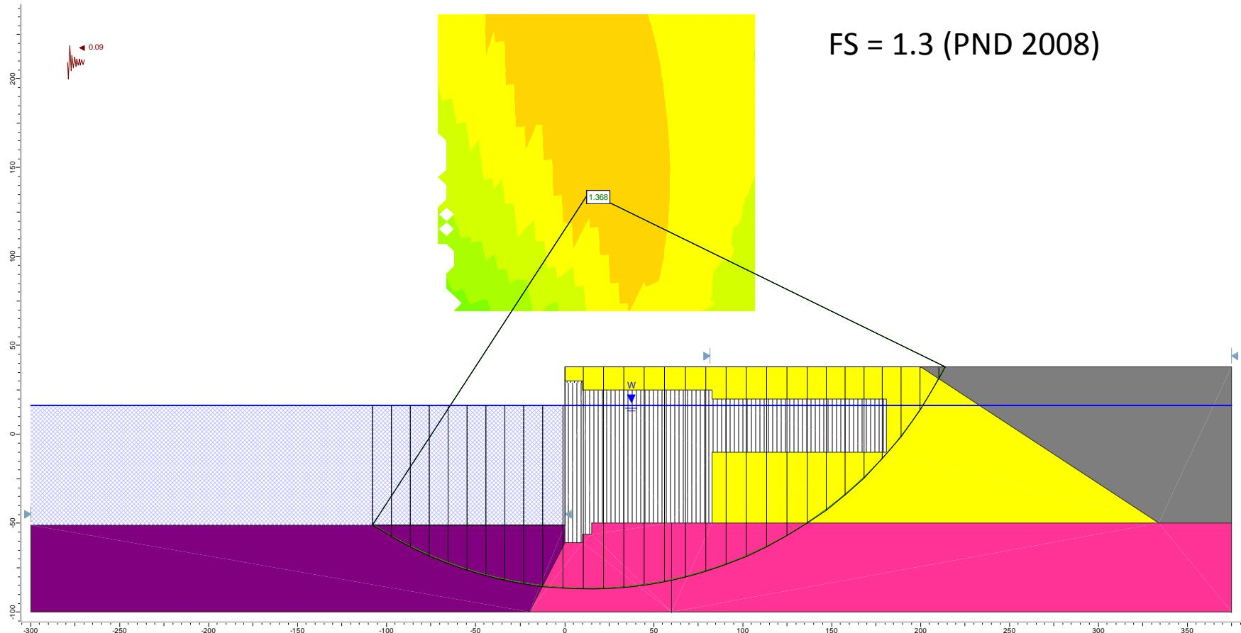
**Figure E39.** Re-analyzing the CLE case for Section F using Slide (2-clay, circular surface).
