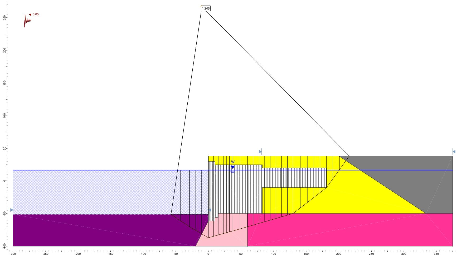
**Figure E34.** Re-analyzing the OLE case for Section F using Slide (3-clay, optimized surface).
