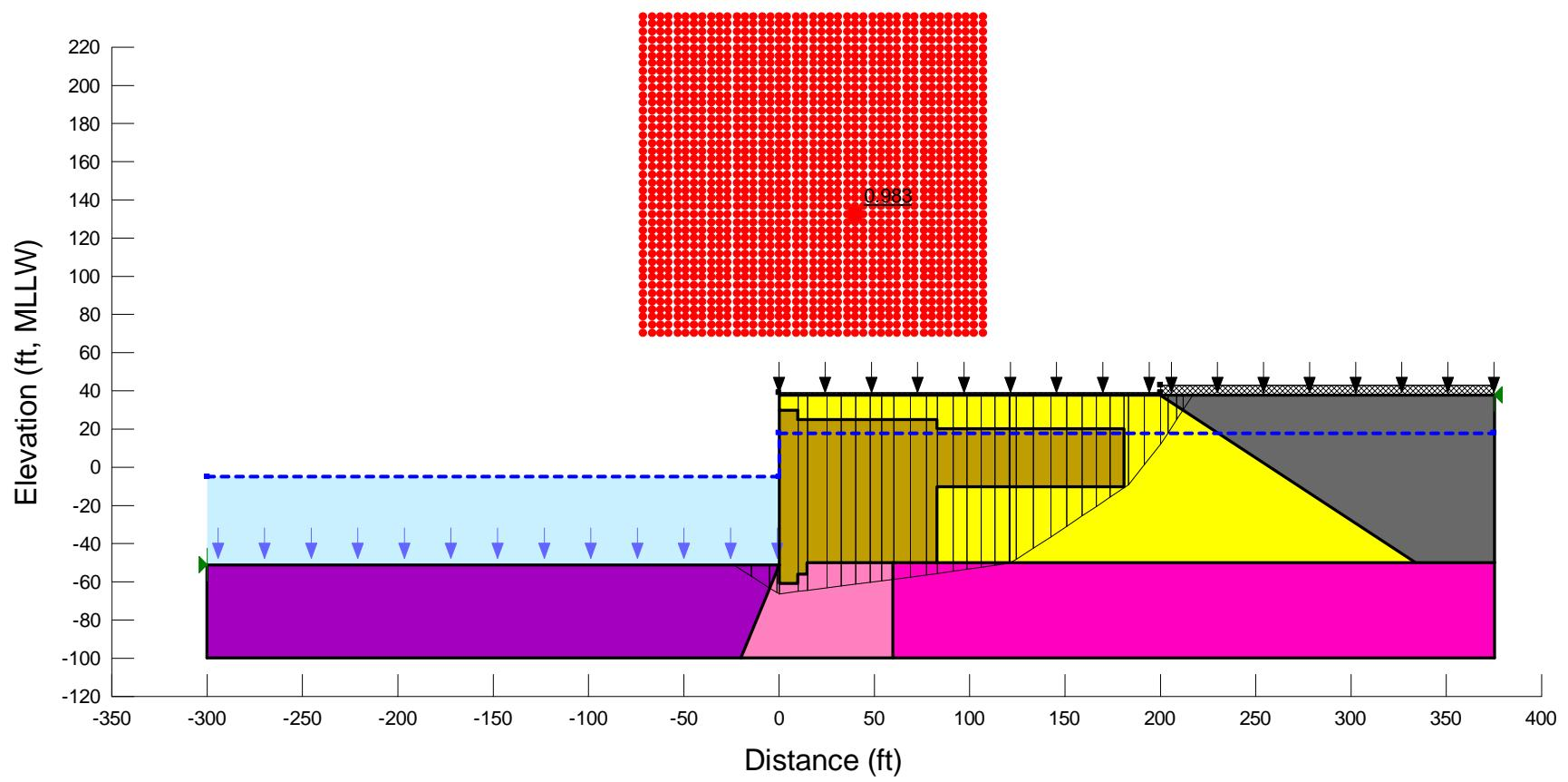
**Figure E14.** Re-analyzing the short-term static (EOC) case for Section F using SLOPE/W (3-clay, optimized surface).
