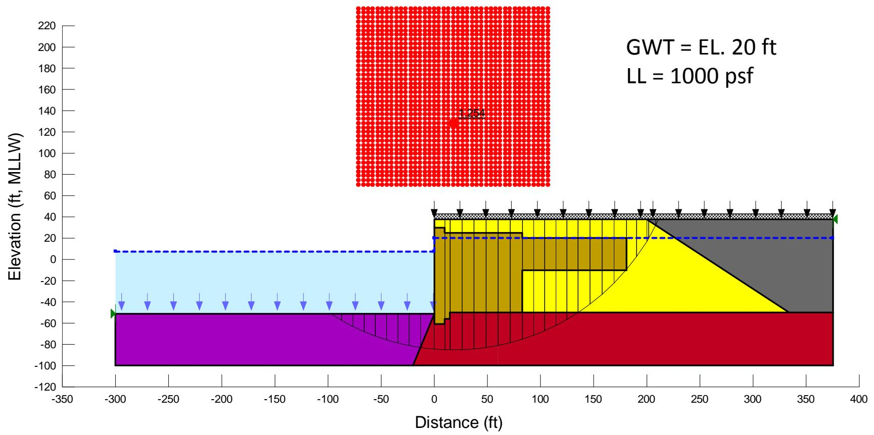
**Figure E53.** Re-analyzing the OLE case for Section F using SLOPE/W (2-clay, circular surface).
