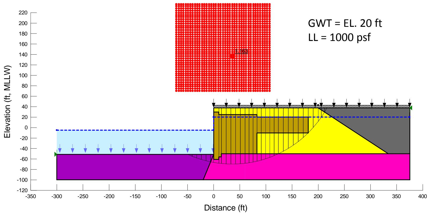
**Figure E51.** Re-analyzing the short-term static (EOC) case for Section F using SLOPE/W (2-clay, circular surface).
