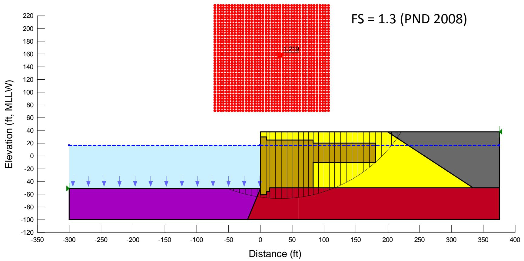
**Figure E35.** Re-analyzing the CLE case for Section F using SLOPE/W (2-clay, circular surface).
