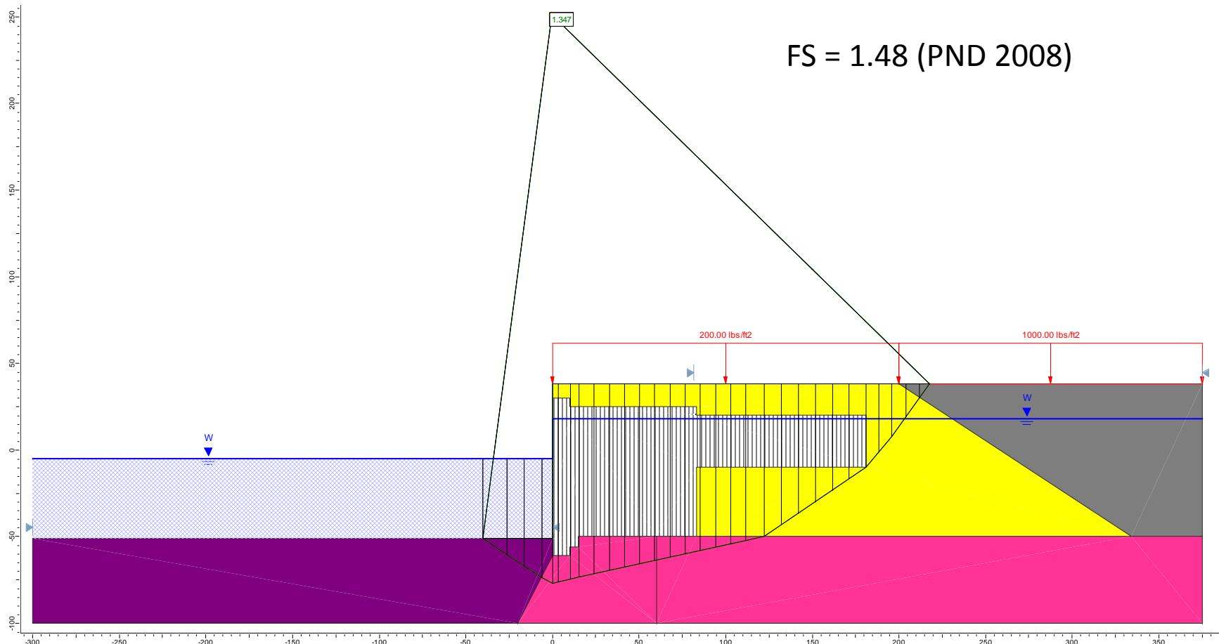
**Figure E24.** Re-analyzing the long-term static-undrained case for Section F using Slide (2-clay, optimized surface).
