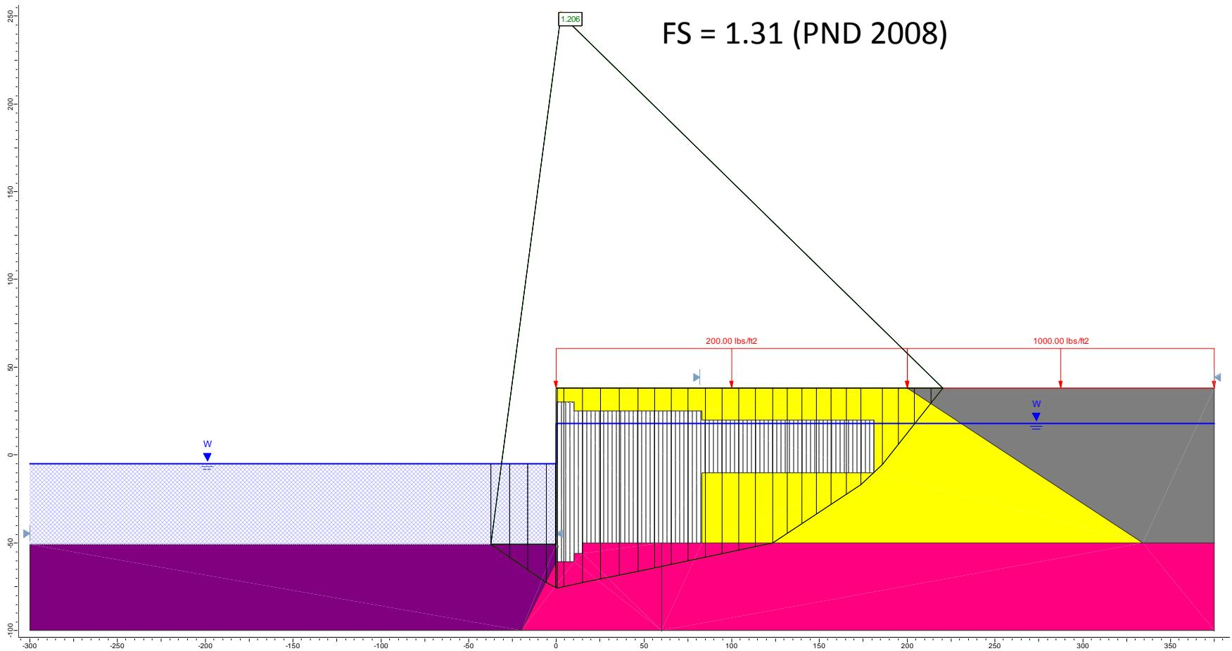
**Figure E16.** Re-analyzing the short-term static (EOC) case for Section F using Slide (2-clay, optimized surface).
