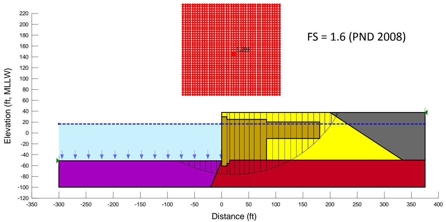
**Figure E27.** Re-analyzing the OLE case for Section F using SLOPE/W (2-clay, circular surface).
