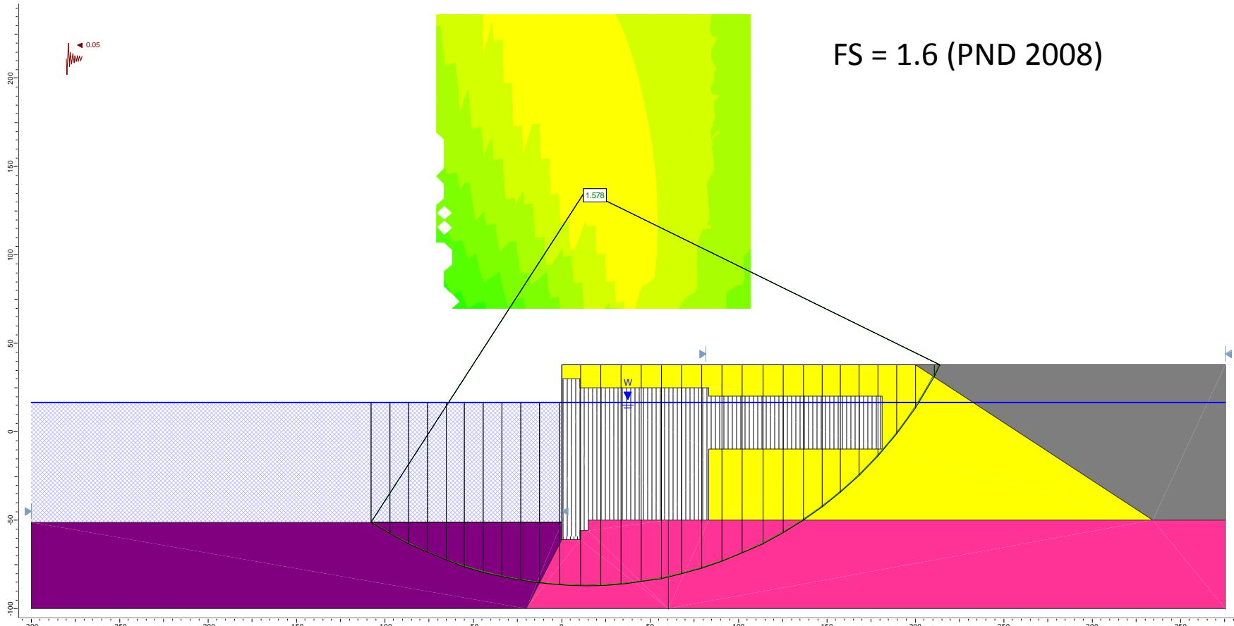
**Figure E31.** Re-analyzing the OLE case for Section F using Slide (2-clay, circular surface).
