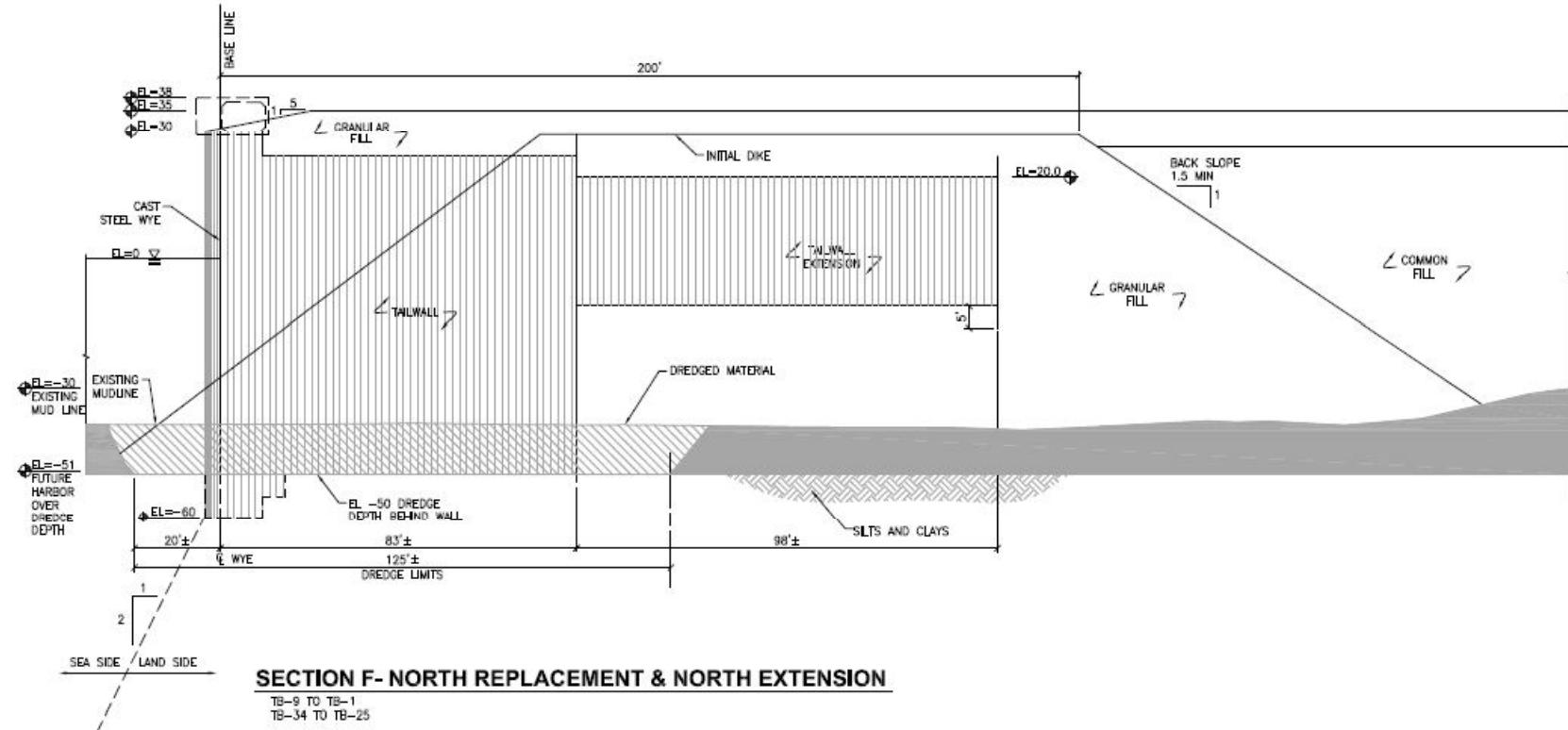
Figure E5. Geometry of Section F (PND, 2008).
