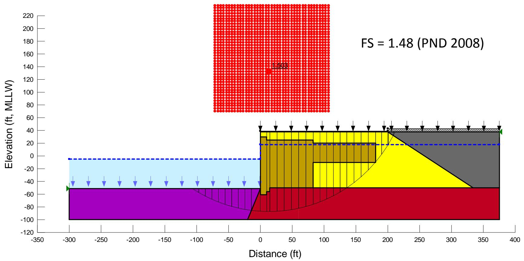
**Figure E19.** Re-analyzing the long-term static-undrained case for Section F using SLOPE/W (2-clay, circular surface).
