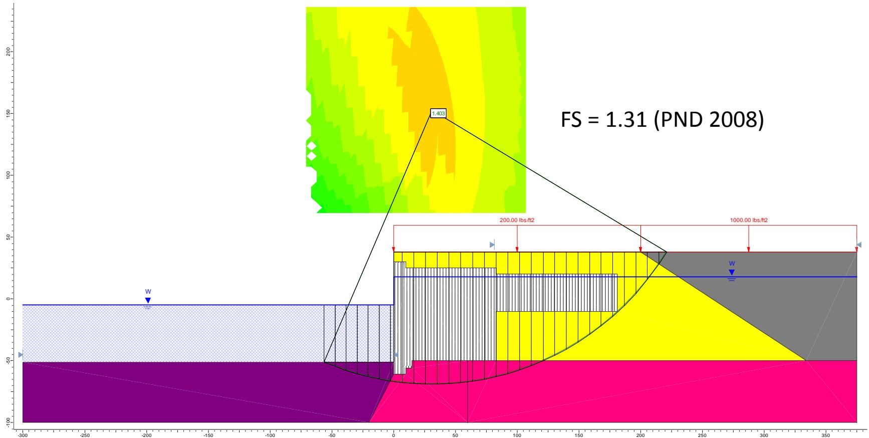
**Figure E15.** Re-analyzing the short-term static (EOC) case for Section F using Slide (2-clay, circular surface).
