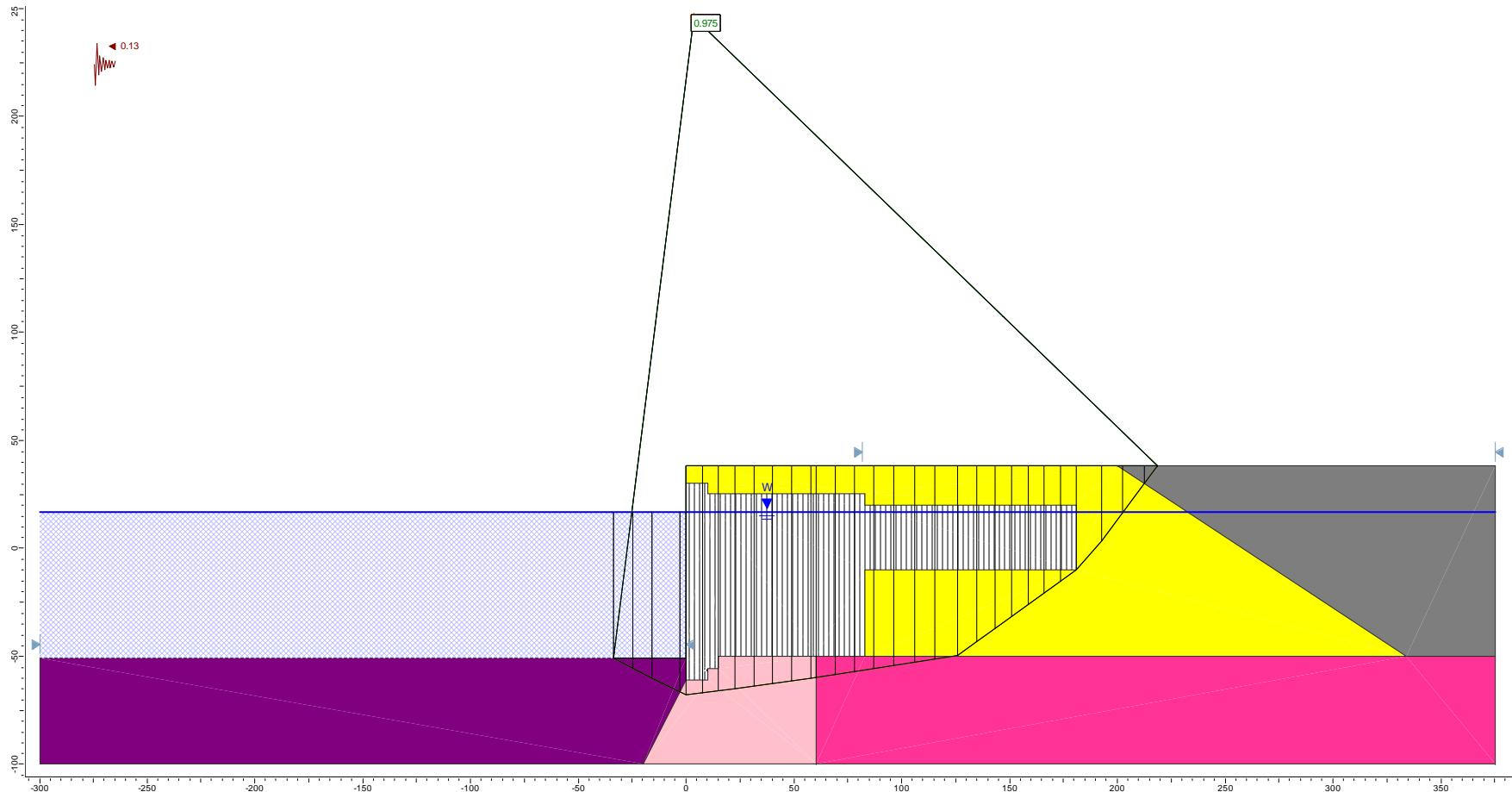
**Figure E50.** Re-analyzing the MCE case for Section F using Slide (3-clay, optimized surface).
