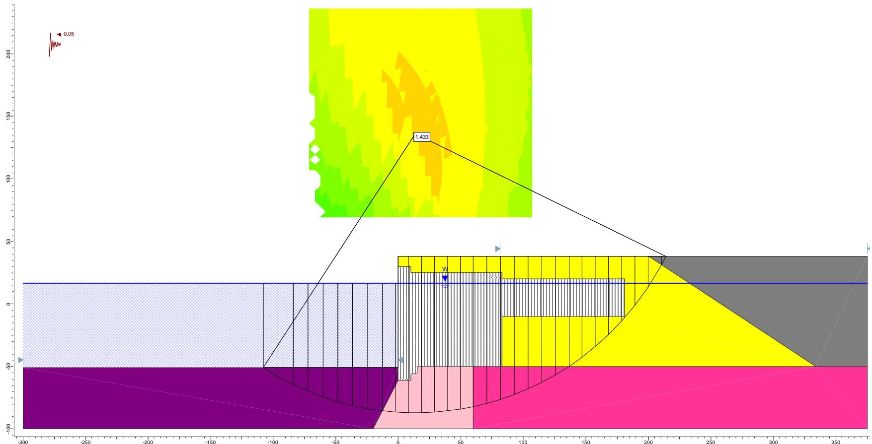
**Figure E33.** Re-analyzing the OLE case for Section F using Slide (3-clay, circular surface).
