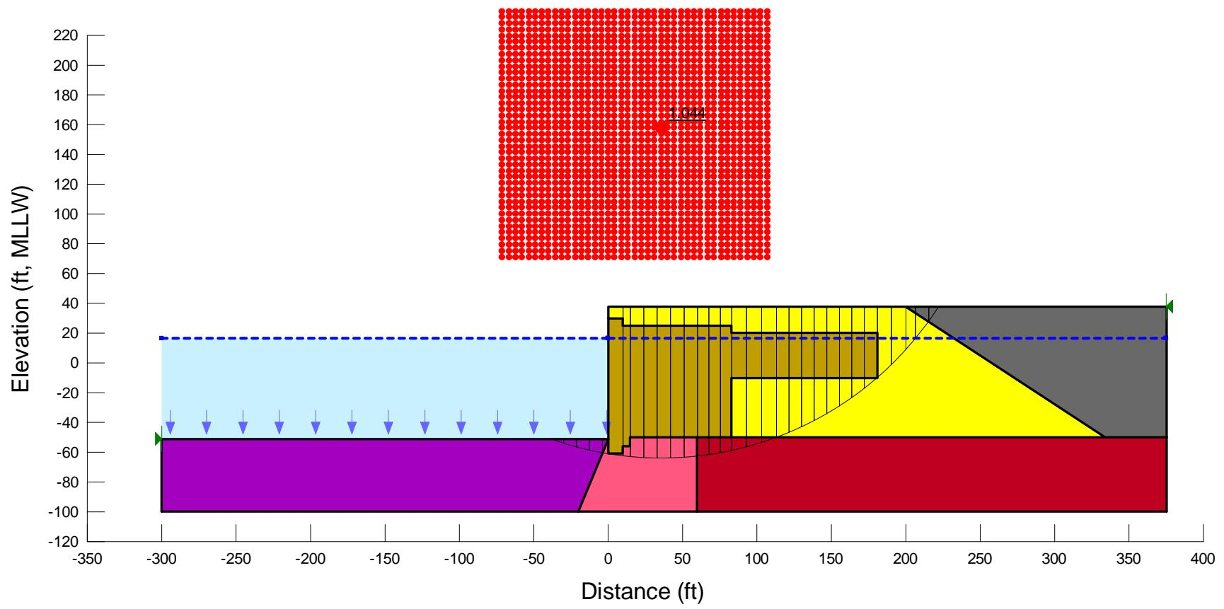
**Figure E38.** Re-analyzing the CLE case for Section F using SLOPE/W (3-clay, optimized surface).
