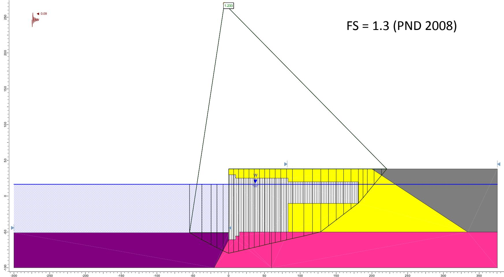
**Figure E40.** Re-analyzing the CLE case for Section F using Slide (2-clay, optimized surface).
