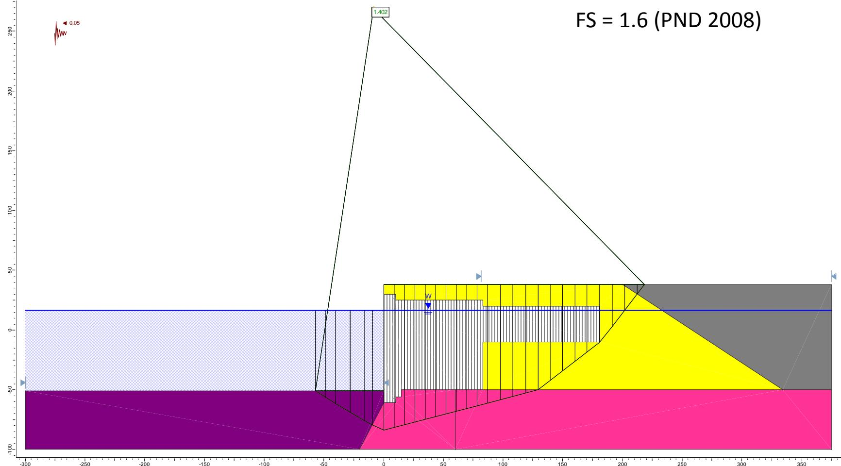
**Figure E32.** Re-analyzing the OLE case for Section F using Slide (2-clay, optimized surface).
