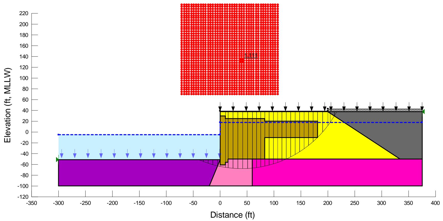
**Figure E13.** Re-analyzing the short-term static (EOC) case for Section F using SLOPE/W (3-clay, circular surface).
