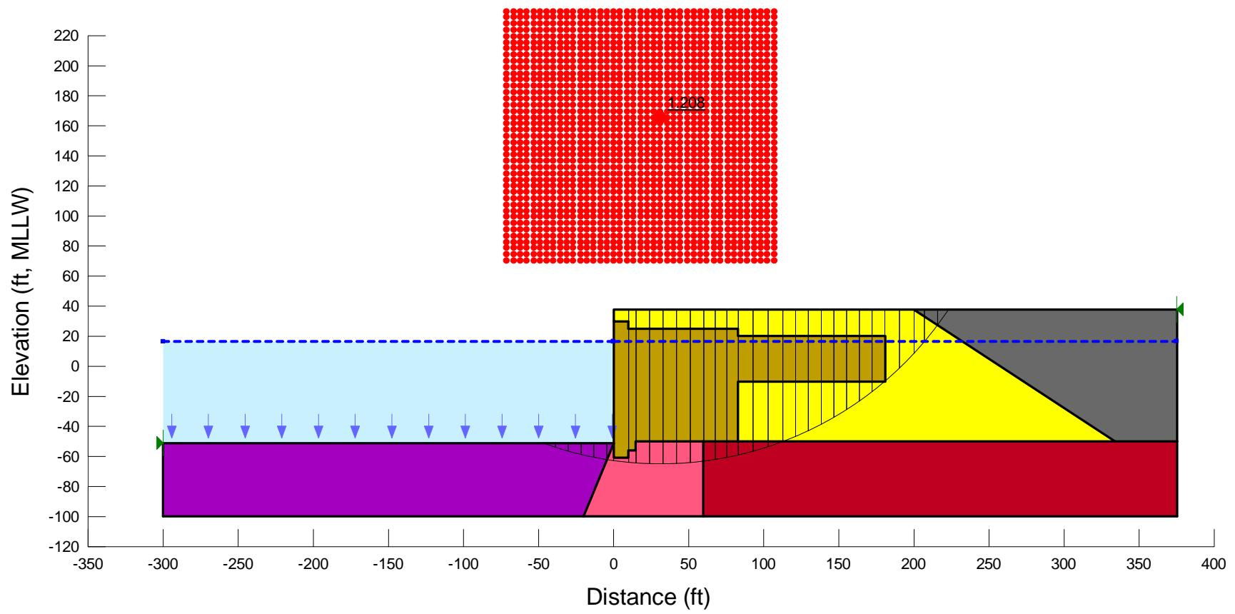
**Figure E29.** Re-analyzing the OLE case for Section F using SLOPE/W (3-clay, circular surface).
