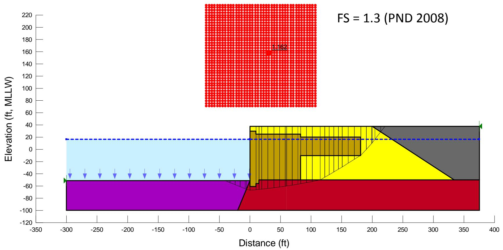
**Figure E36.** Re-analyzing the CLE case for Section F using SLOPE/W (2-clay, optimized surface).
