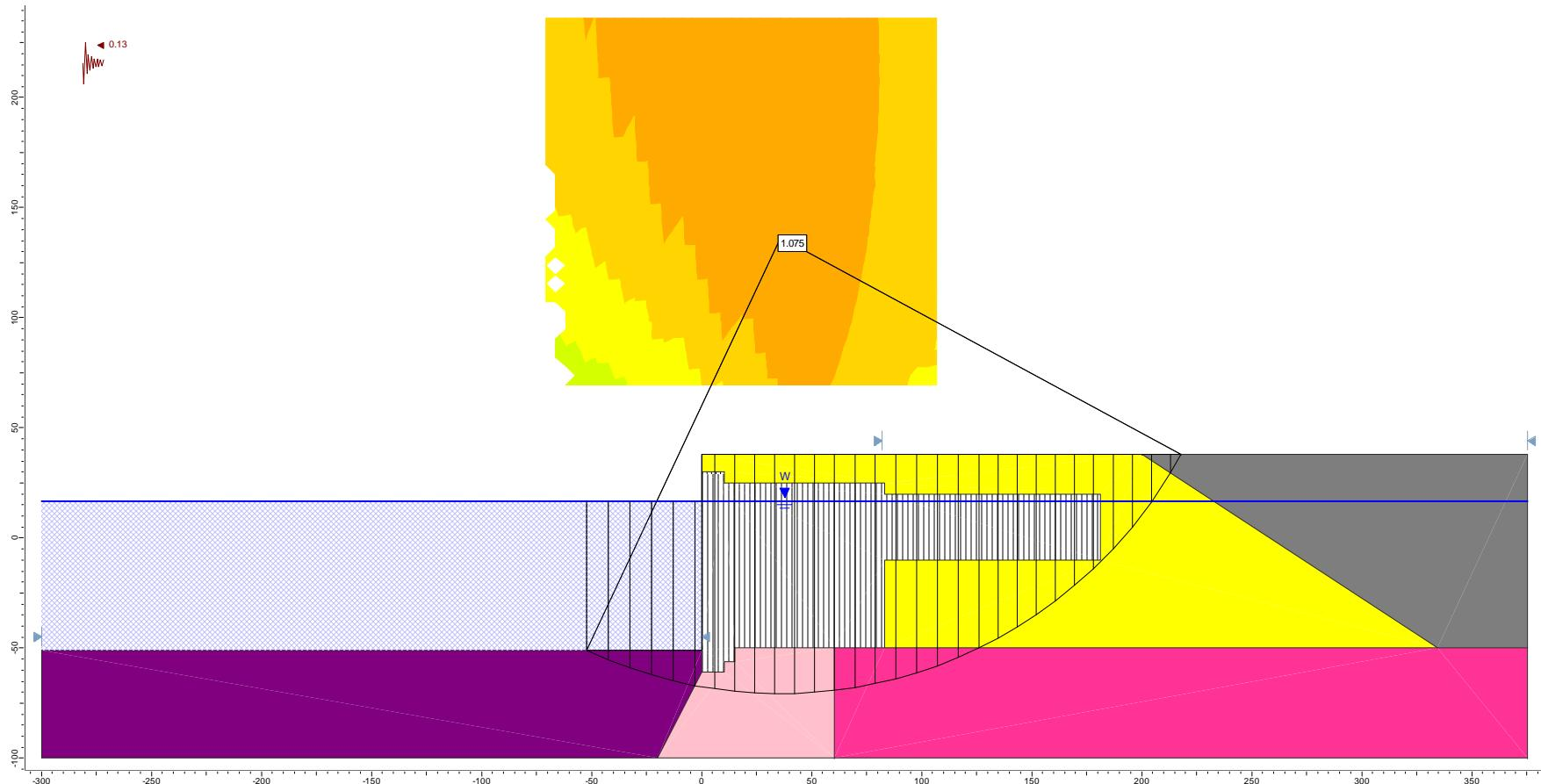
**Figure E49.** Re-analyzing the MCE case for Section F using Slide (3-clay, circular surface).
