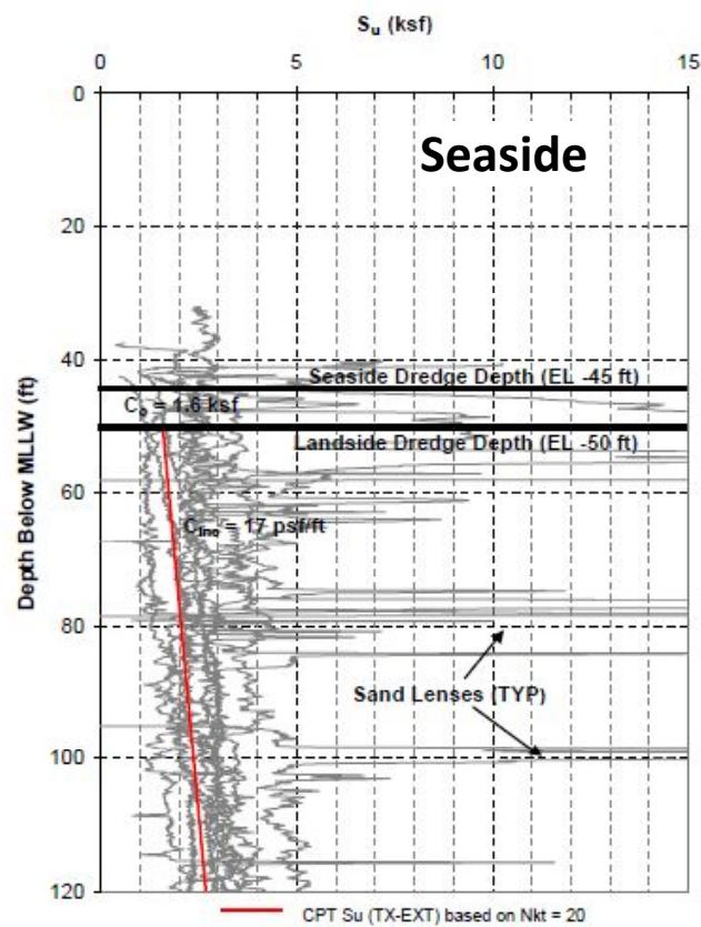
Figure 4.23 Undrained-Shear Strength Profile from CPT (TX-E) Short-Term Static, Long-Term Static, and Seismic Conditions for Analysis Section F
