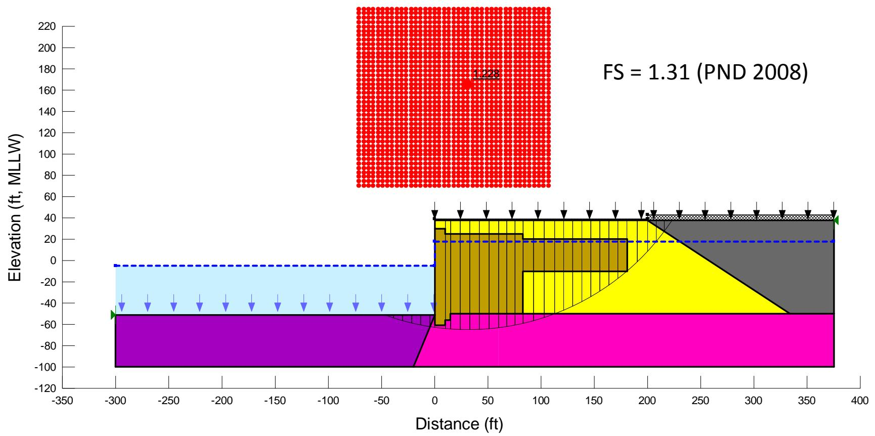
**Figure E11.** Re-analyzing the short-term static (EOC) case for Section F using SLOPE/W (2-clay, circular surface).
