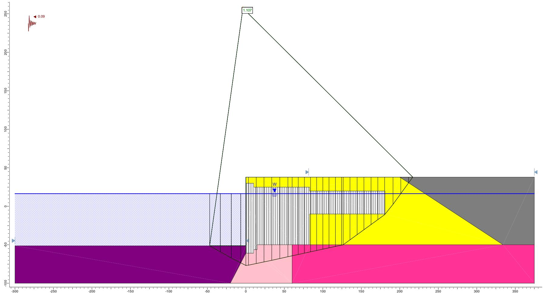
**Figure E42.** Re-analyzing the CLE case for Section F using Slide (3-clay, optimized surface).
