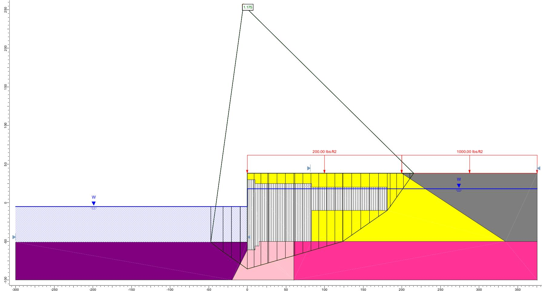
**Figure E26.** Re-analyzing the long-term static-undrained case for Section F using Slide (3-clay, optimized surface).
