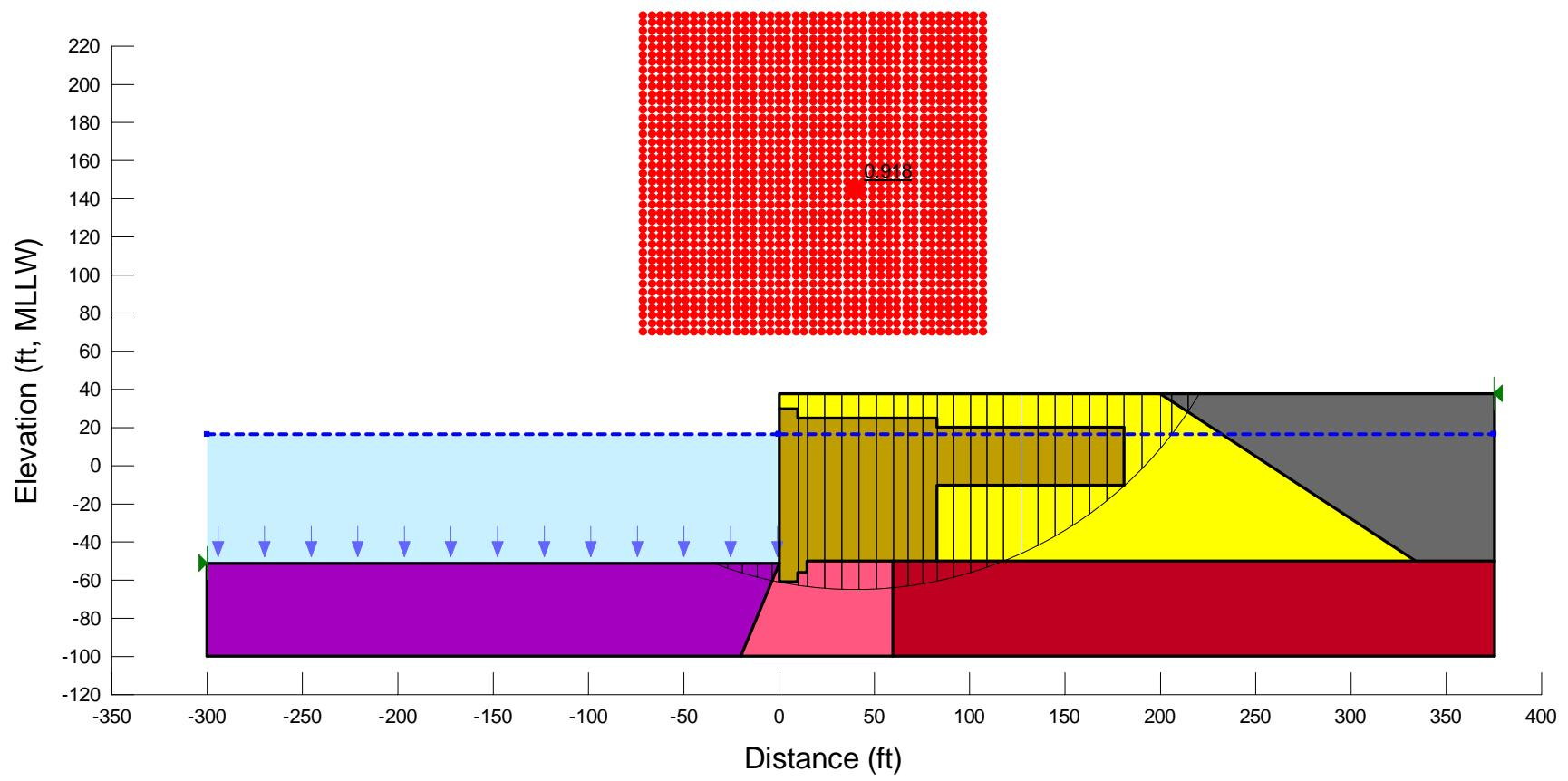
**Figure E45.** Re-analyzing the MCE case for Section F using SLOPE/W (3-clay, circular surface).
