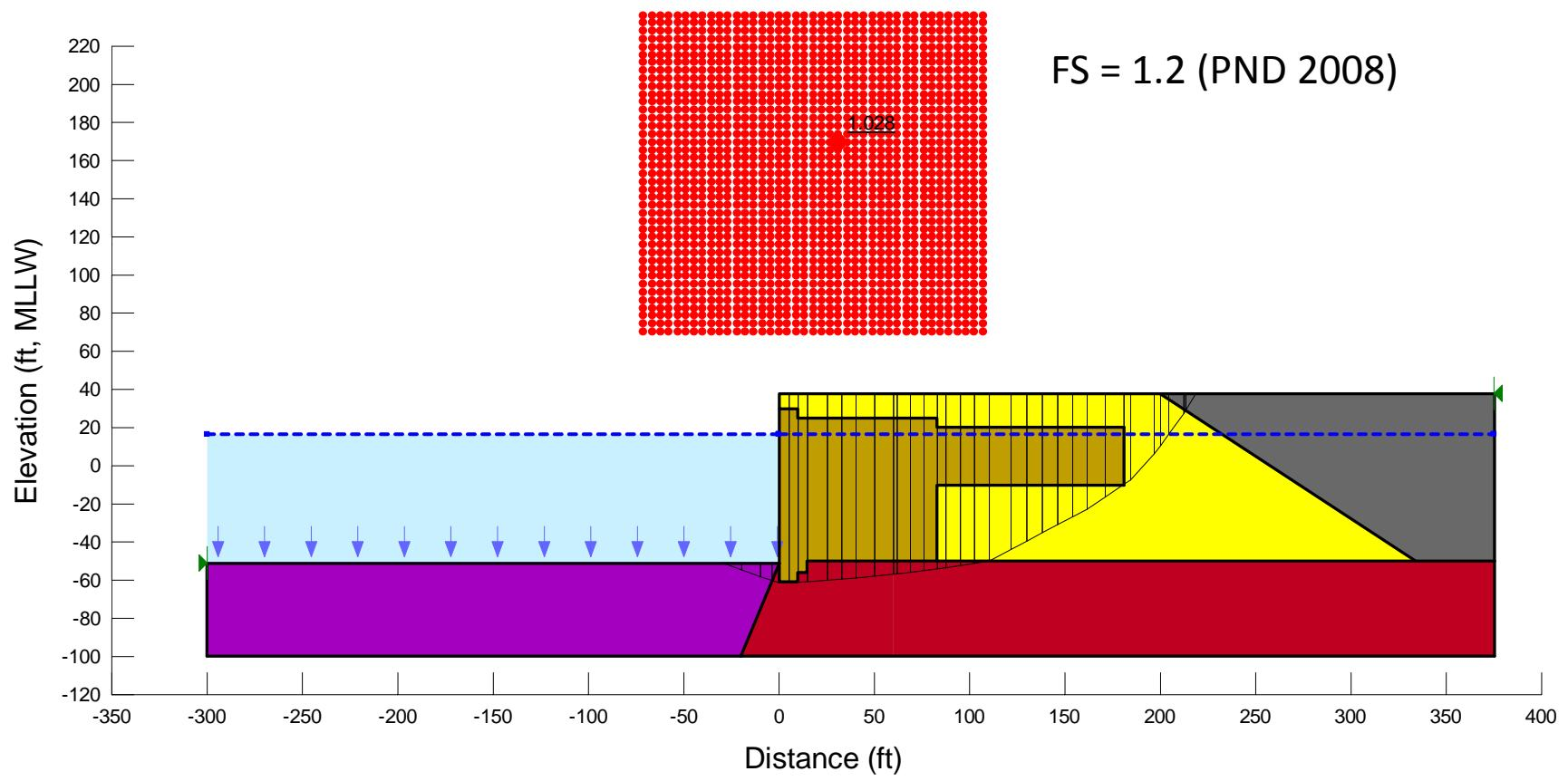
**Figure E44.** Re-analyzing the MCE case for Section F using SLOPE/W (2-clay, optimized surface).
