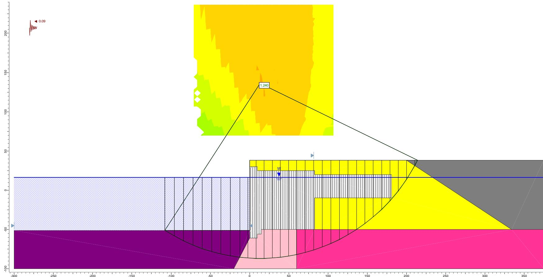
**Figure E41.** Re-analyzing the CLE case for Section F using Slide (3-clay, circular surface).
