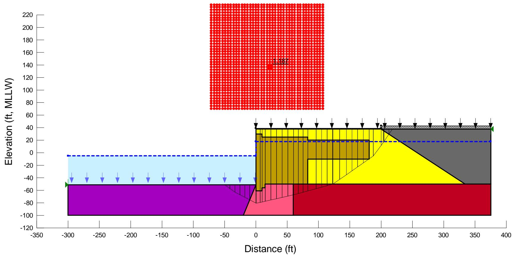
**Figure E22.** Re-analyzing the long-term static-undrained case for Section F using SLOPE/W (3-clay, optimized surface).
