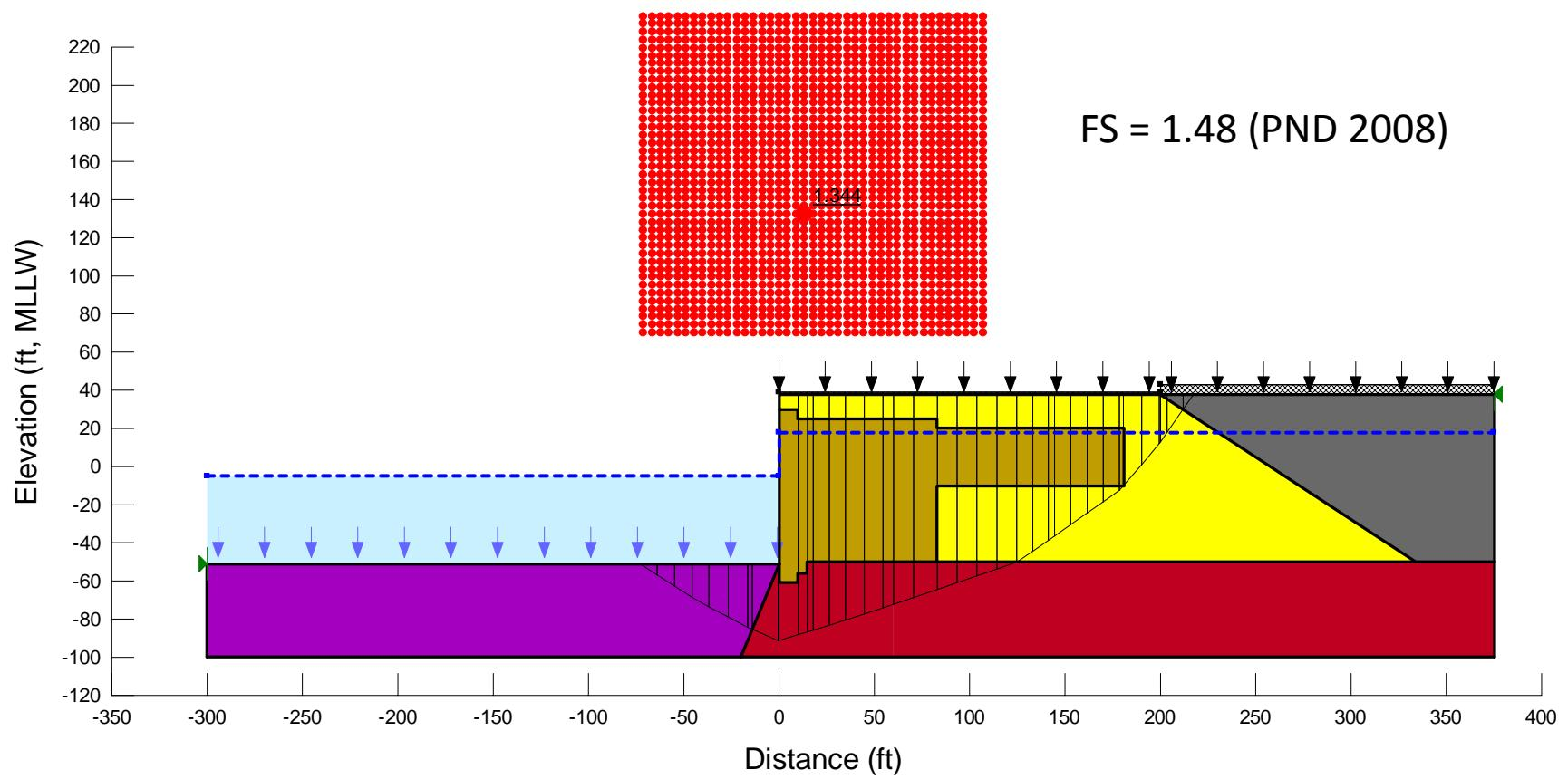
**Figure E20.** Re-analyzing the long-term static-undrained case for Section F using SLOPE/W (2-clay, optimized surface).
