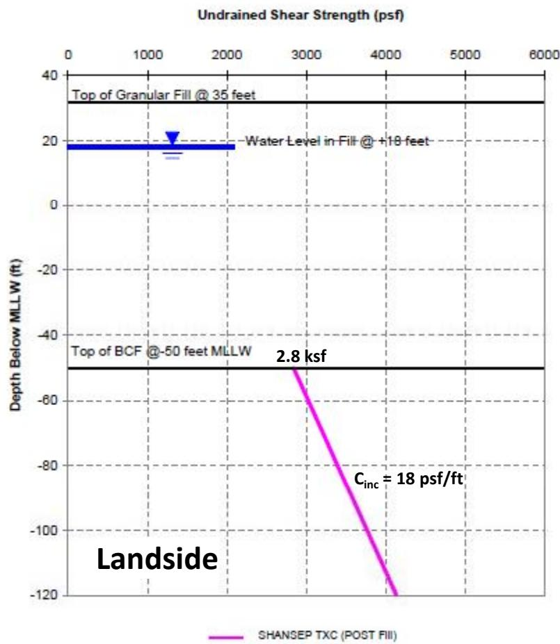
Figure 4.30 Undrained-Shear Strength Profile Based on SHANSEP-TXC Equation – Long-Term Static and Seismic Conditions for Analysis Section F
