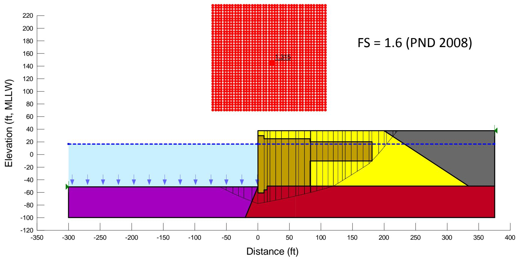
**Figure E28.** Re-analyzing the OLE case for Section F using SLOPE/W (2-clay, optimized surface).
