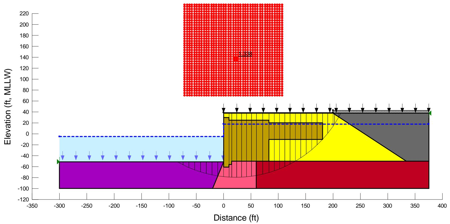
**Figure E21.** Re-analyzing the long-term static-undrained case for Section F using SLOPE/W (3-clay, circular surface).
