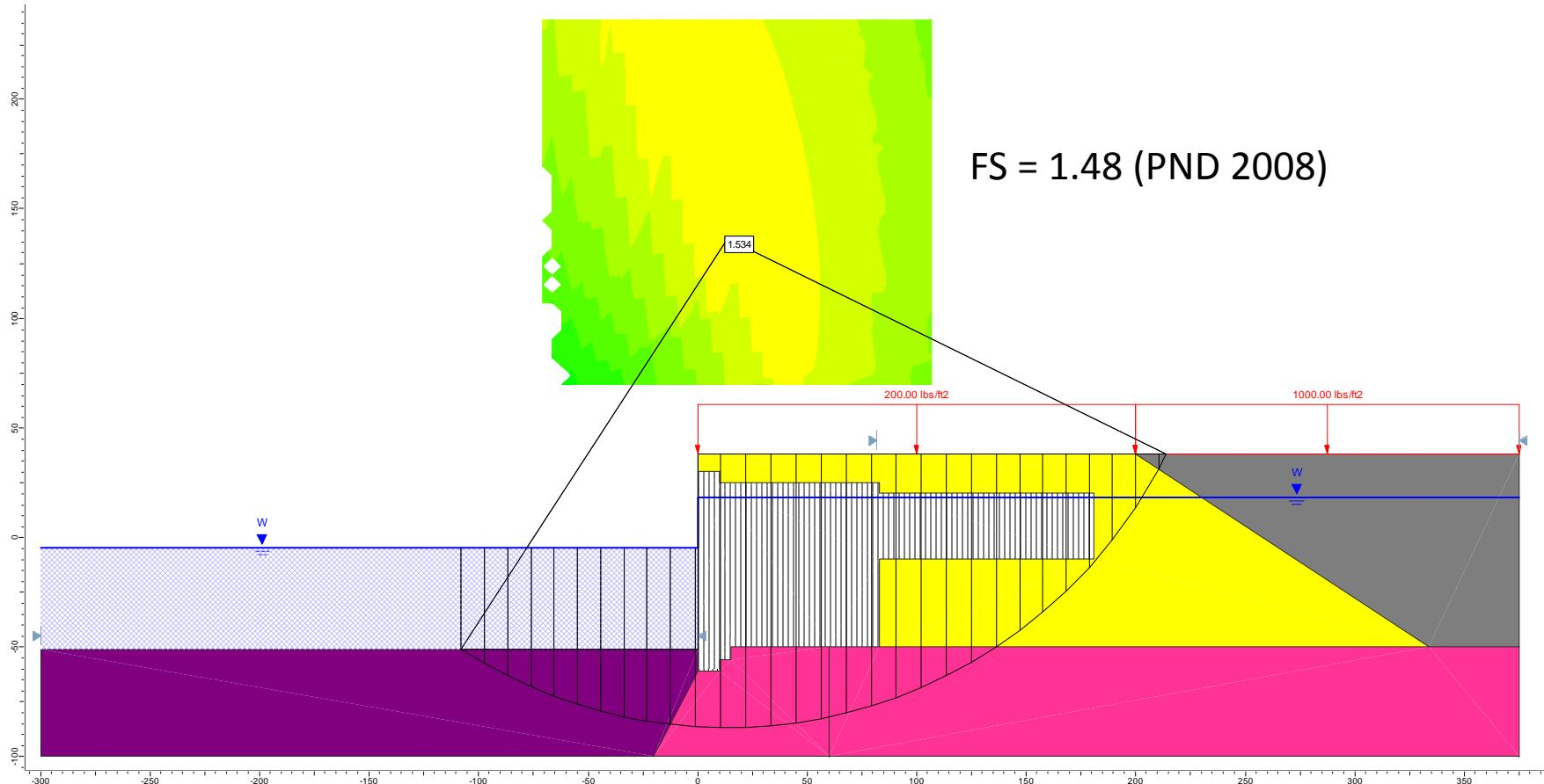
**Figure E23.** Re-analyzing the long-term static-undrained case for Section F using Slide (2-clay, circular surface).
