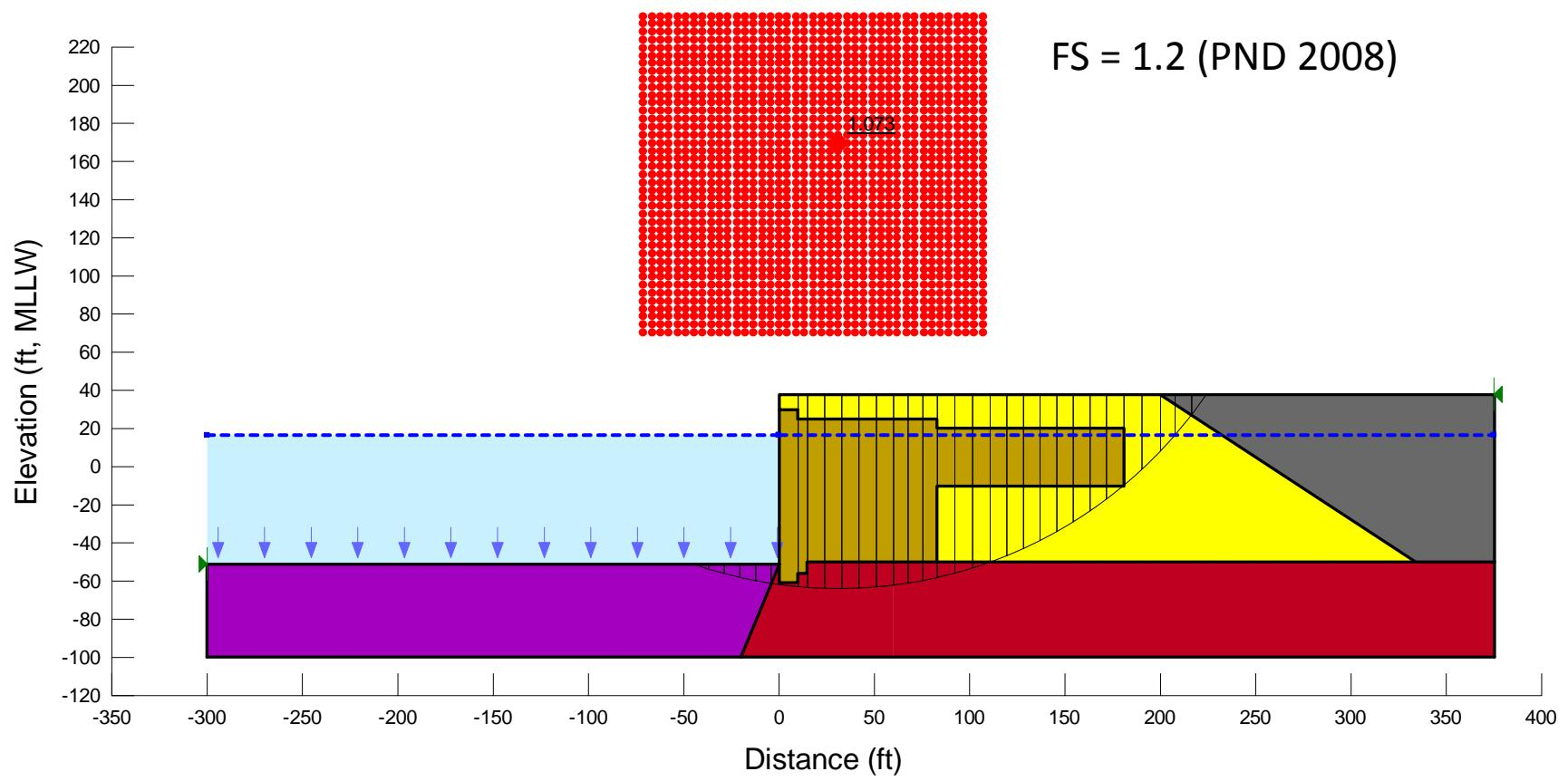
**Figure E43.** Re-analyzing the MCE case for Section F using SLOPE/W (2-clay, circular surface).
