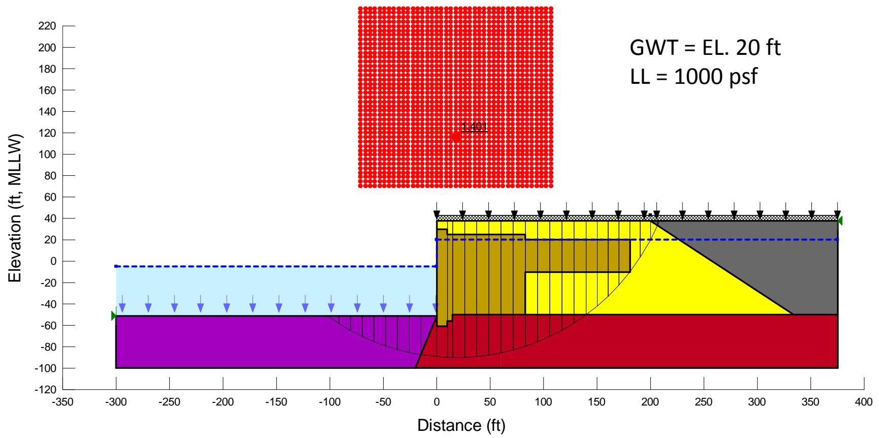
**Figure E52.** Re-analyzing the long-term static case for Section F using SLOPE/W (2-clay, circular surface).
