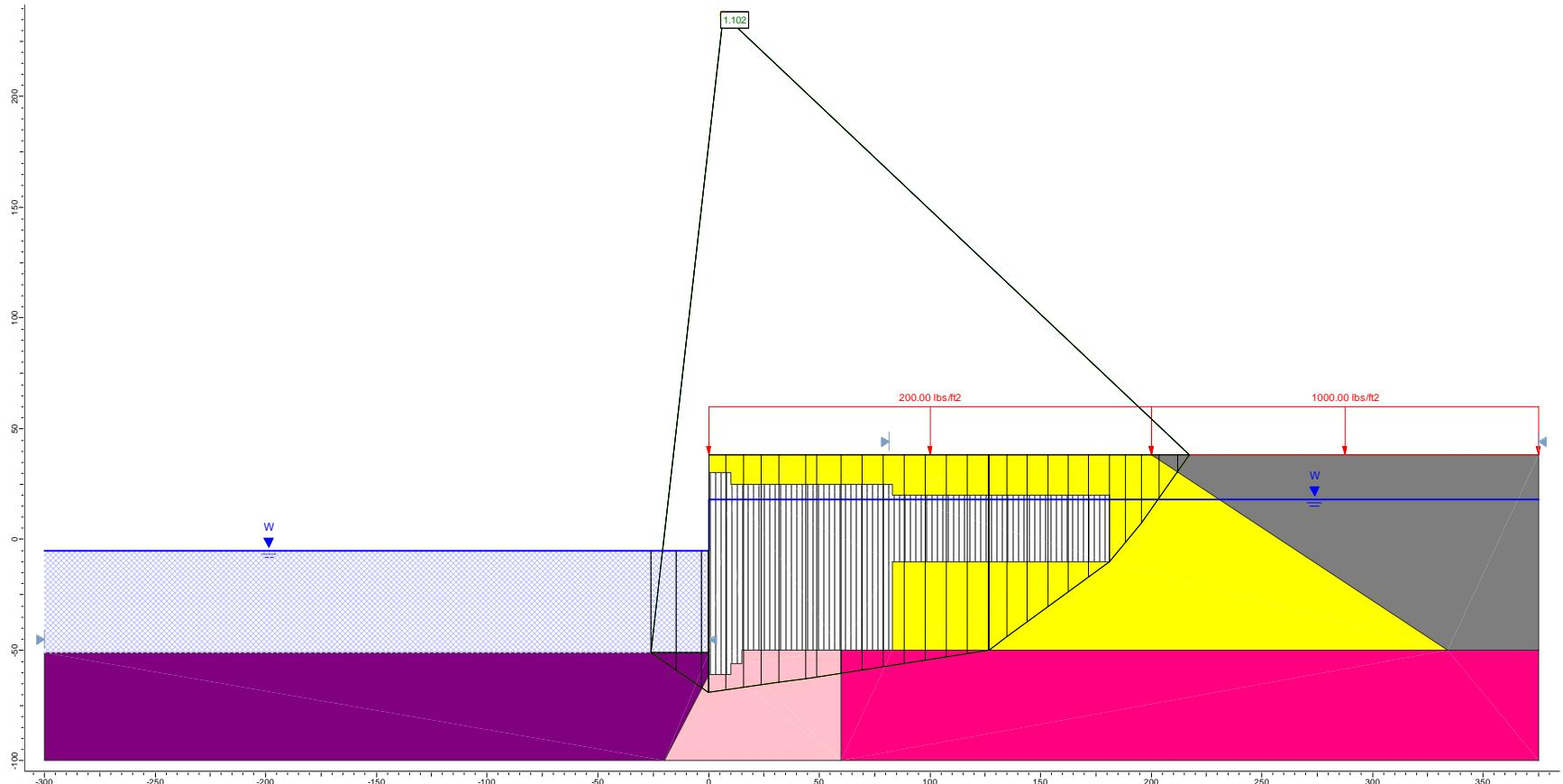
**Figure E18.** Re-analyzing the short-term static (EOC) case for Section F using Slide (3-clay, optimized surface).
