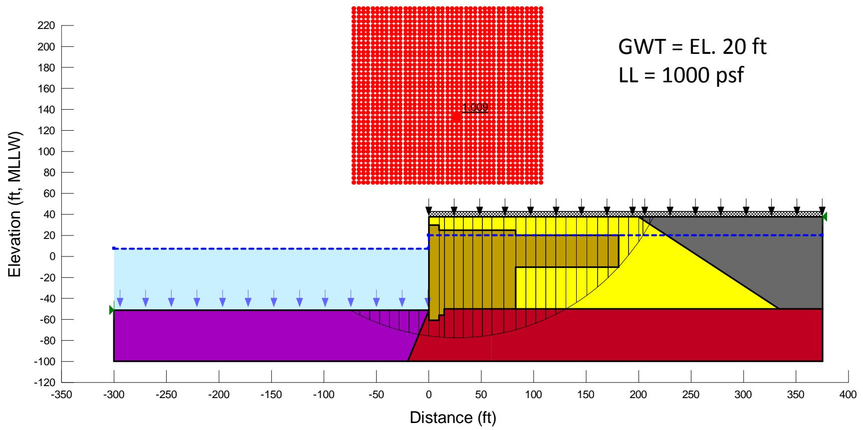
**Figure E55.** Re-analyzing the MCE case for Section F using SLOPE/W (2-clay, circular surface).
