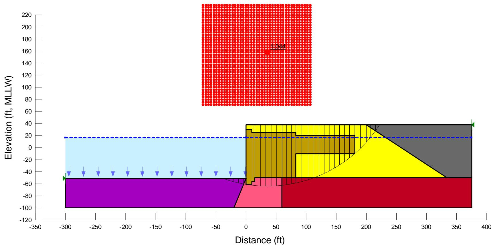
**Figure E37.** Re-analyzing the CLE case for Section F using SLOPE/W (3-clay, circular surface).
