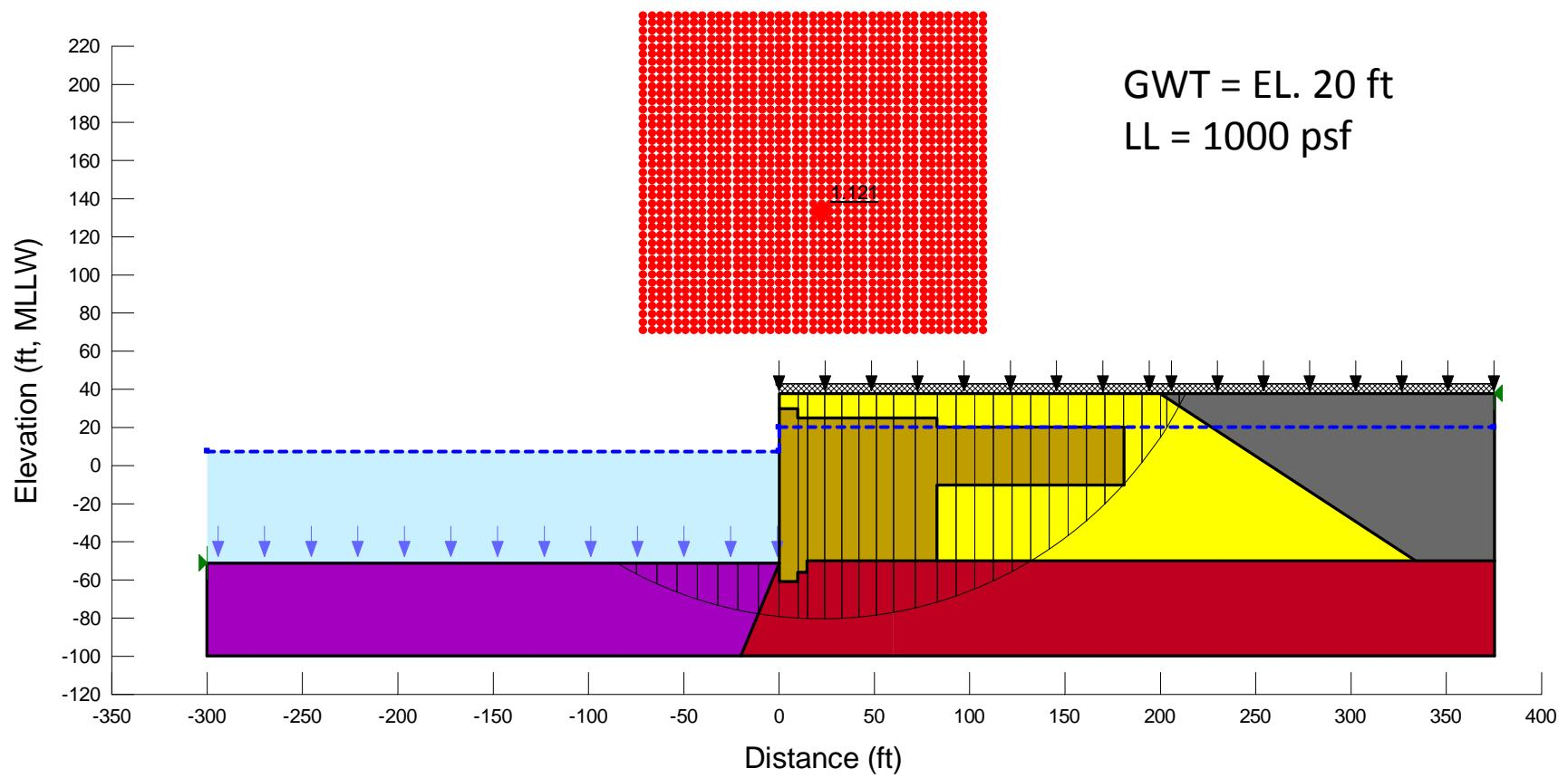
Figure E54. Re-analyzing the CLE case for Section F using SLOPE/W (2-clay, circular surface).
