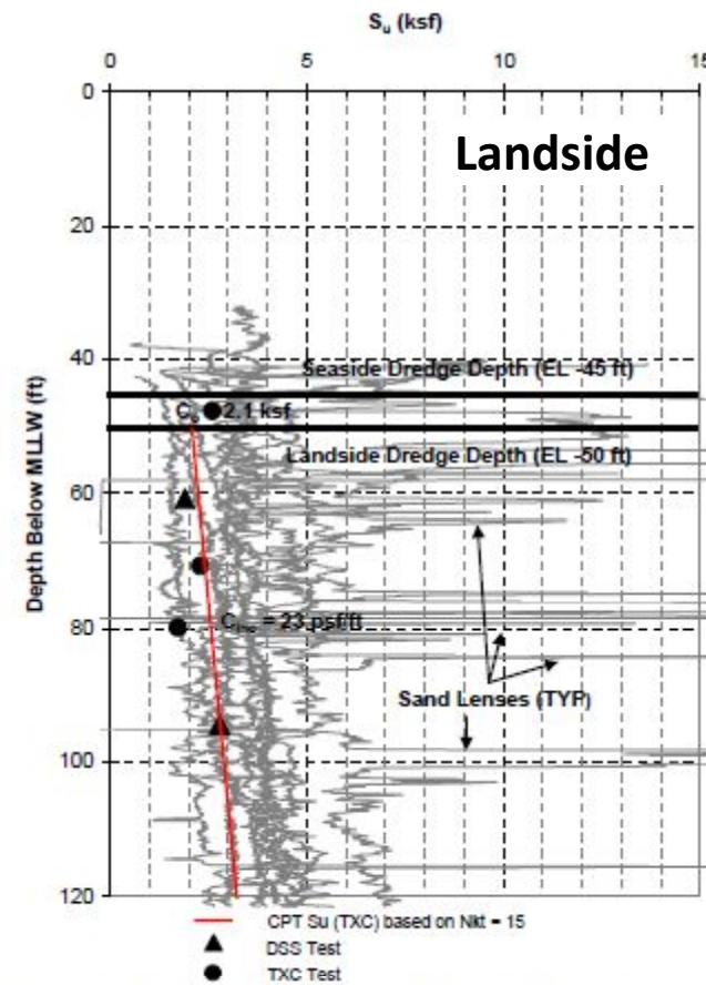
Figure 4.17 Undrained-Shear Strength Profile from CPT (TXC) Short-Term Static Conditions for Analysis Section F
