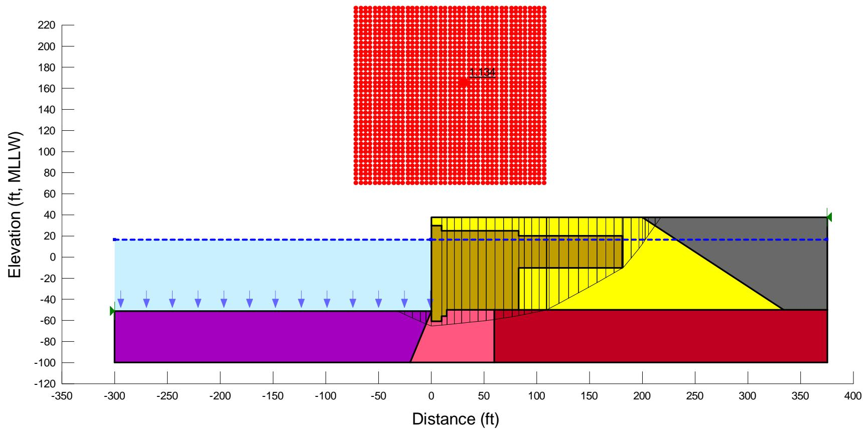
**Figure E30.** Re-analyzing the OLE case for Section F using SLOPE/W (3-clay, optimized surface).
